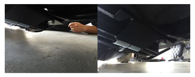
Now insert the bolt thru the hole in the center stand and screw it into the welded nut on J bracket use a 3/4" socket to tighten up the bolt.
