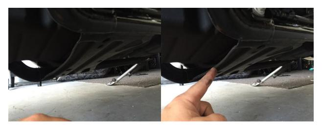
2).locate the J Bracket with the welded nut on it remove the bolt and place over frame on left side lining up the hole from the nut on the J bracket with the hole on the crossbar
