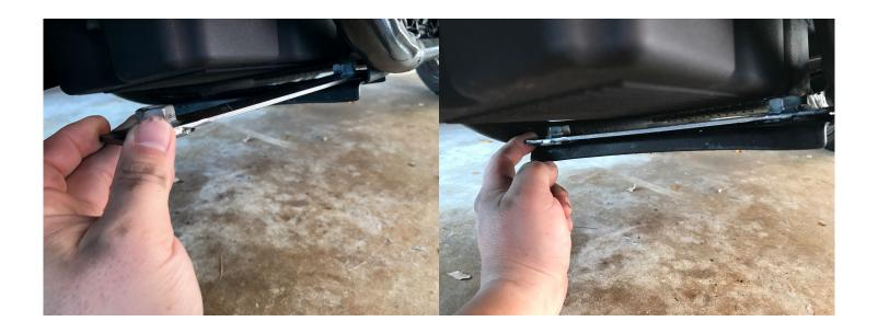
4.) Slide the center Stand underneath the frame crossbar with the foot push down lever on the left side of the bike (kickstand side) and simply line up the 2 holes on the center stand with the 2 holes on the frame crossbar and lock crossbar once all the holes are lined up use the 2 provided bolts and lock washers with a 3/4" socket to bolt down the center stand to the bike.
