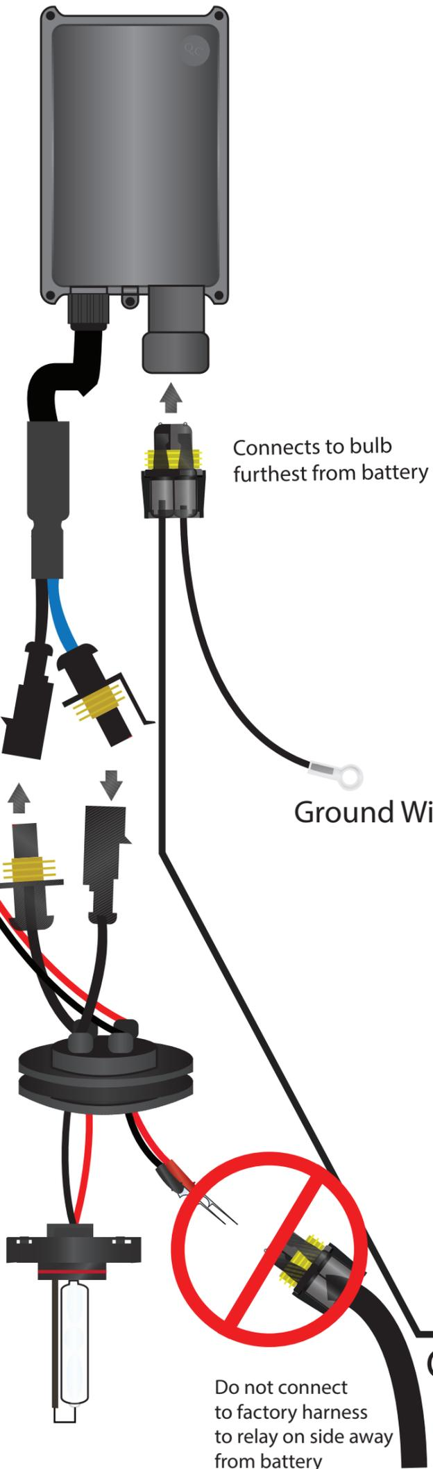
Connects to bulb furthest from battery
