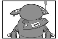
C. Remove the Screws from the blade holder and keep it aside.
