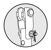
IMPORTANT: Must check LOCK PIN is inserted and SPREAD OPEN with PLIERS.
