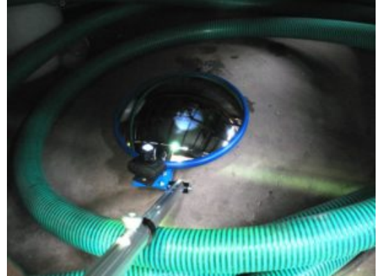
3000mm Heavy Duty 'Look Under' Inspection Mirror with Light
