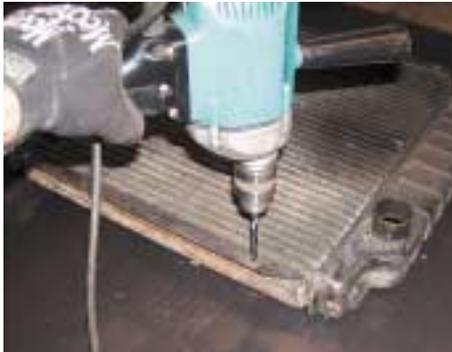
Step 1: After removing the radiator, drill out the stock mounting nuts with a 5/16" drill bit.
