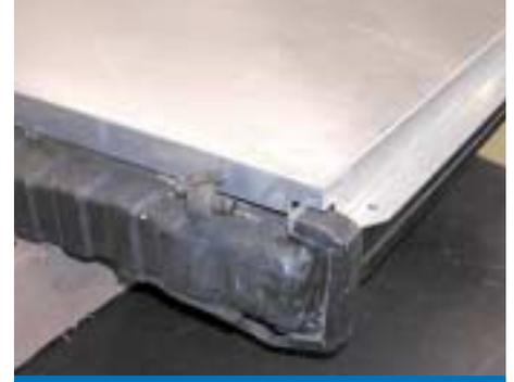
Step 5: cut out notches for stock mounting brackets (if needed).
