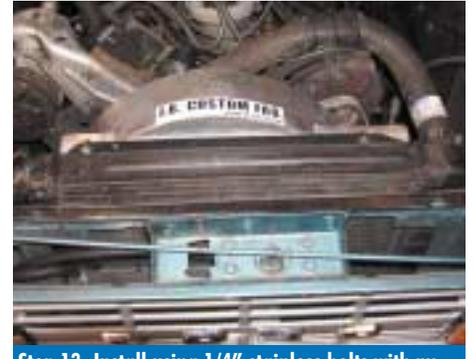
**Step 13: Install using 1/4" stainless bolts with ny-lock nuts.**
