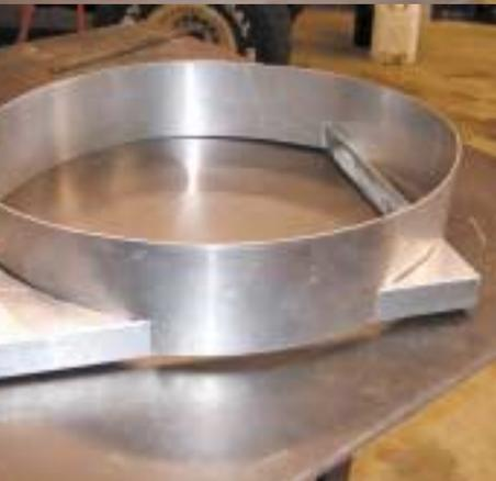
**Step 10: Cut slits in the barrel to allow the barrel to slide over the box.**
