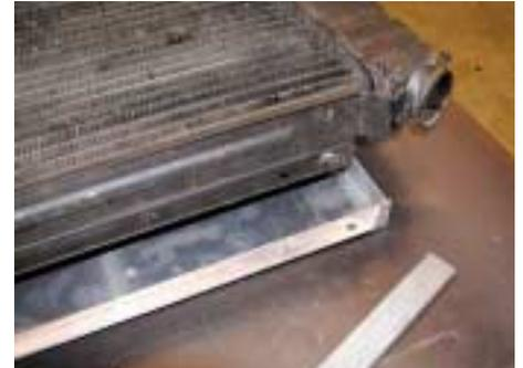
Step 4: Drill 5/16" mounting holes and cut corners of shroud mounting flange to match the flange on the radiator.
