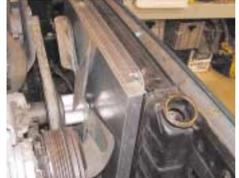
Step 6: With radiator in place mark the center of the fan on the box.
