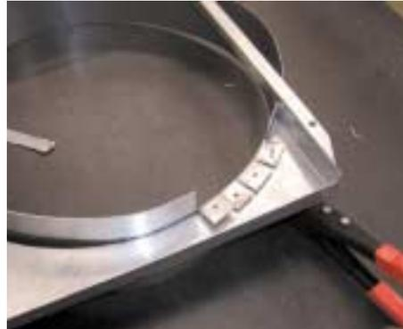
**Step 11a (the cheap method): Attach barrel to box.**
