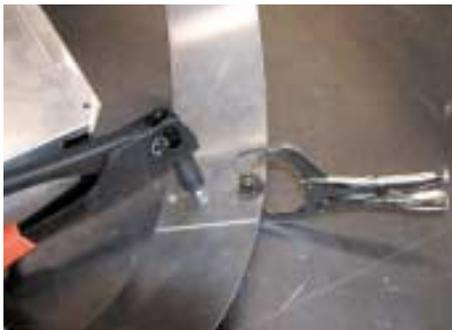
**Step 9: After deciding how much of the fan to cover, create the barrel of the shroud by coiling a strip of aluminum to fit the hole in the box.**
