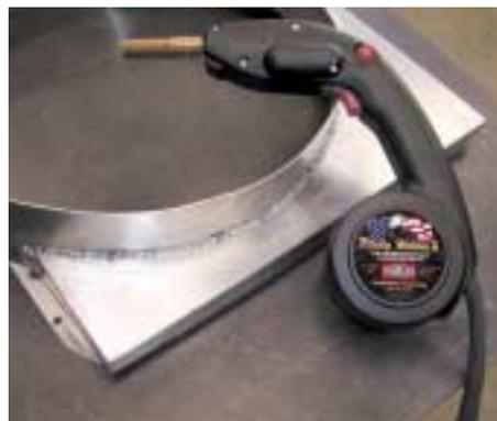
**Step 11b (the easy method): Attach barrel to box. Yes...that was done with a Ready Welder!**
