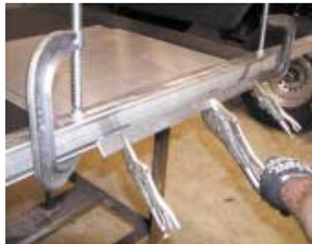
Step 3a (the cheap method): Bend into box.
