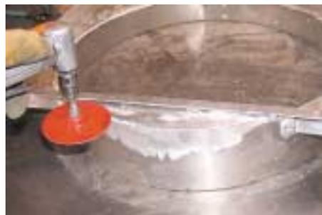
**Step 12: close up the air gaps where the barrel is outside of the dimensions of the box, and remove most of the box that is inside of the barrel (so the air can flow through and the fan will not hit the inside of the box).**
