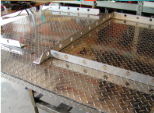
31 The bottom and lid of the box were reinforced with 2" X 2" 3/16" aluminum angle ribs to keep the top from flexing and to provide a mounting point for the folding leg that would support the top when open.
