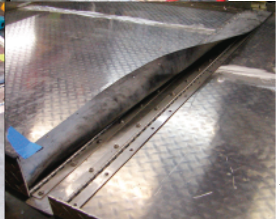
30 A seal was made for the hinged end of the box to keep out the rain sand from 1/8" EPDM gasket material.
