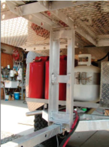
28 The box would fold out toward the front of the trailer and be supported by a folding leg that clips to the trailer tongue.
