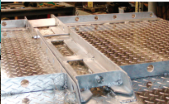
29 make the bottom of the box lay flat when opened two stainless piano hinges were used and attached with counter-sunk 1/4" stainless steel socket head machine screws.
