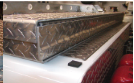
30 A seal was made for the hinged end of the box to keep out the rain sand from 1/8" EPDM gasket material.
