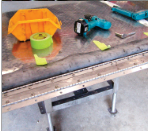
29 make the bottom of the box lay flat when opened two stainless piano hinges were used and attached with counter-sunk 1/4" stainless steel socket head machine screws.
