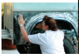
The trailer was now transported to Keizer Collision Center in Keizer, OR, were my wife applied the gravel guard to the front of the fenders and flares, (22) and sprayed the tri-coat white with blue pearl paint supplied by Industrial Finishes in Salem OR. Once the paint was cured, it was taken to Mid-valley Line-X of Salem OR, where the inside was sprayed with a liberal coating of urethane bed-liner.
