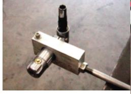
Since air was going to be plumbed to the trailer it just seemed logical to add a blender (you just never know when you will need one on the trail). (19) The blender was modified from a standard home model by replacing the electric motor assembly with an angle head die grinder and some custom bracketry.
