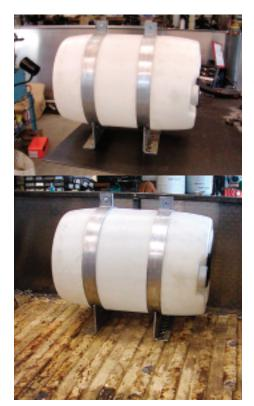
**16** For the water supply a 15-gallon carboy was used, and mounted to the inside of the tub with aluminum straps.
