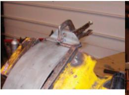
14A tray was fabricated from 1 1/2" .125 304 stainless steel angle, and the mounts added for each of the items. The mounts for the generator were the most challenging, the solution was, using equipment vibration isolation mounts available from McMaster-Carr...
