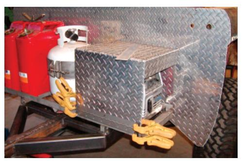
17The water is pumped with a Shurflo 12 volt pump with a built –in pressure switch through a 1/2" poly-braid hose with a hand sprayer that has a quick disconnect on the front bulkhead of the trailer.
