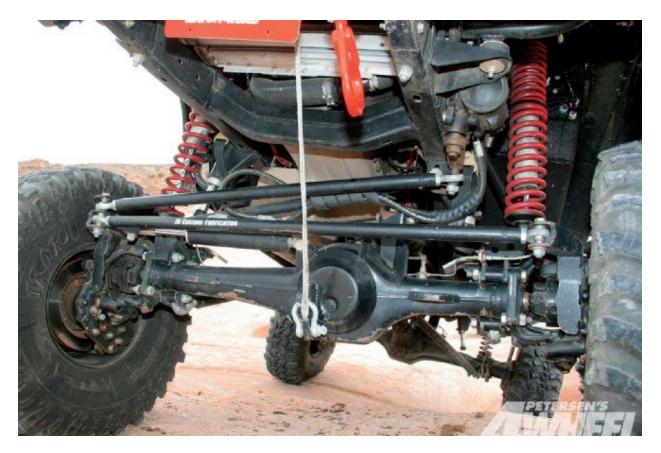
To control the high-clearance 404 Unimog front axle, the Bronco runs a three-link suspension that utilizes a track bar. Since the portal boxes make the Unimog axles substantially taller than a traditional 1-ton axle set, Jon used a set of 16-inch Fox coilovers and bumpstops to create a controlled suspension dynamic capable of performing well in a multitude of environments.
