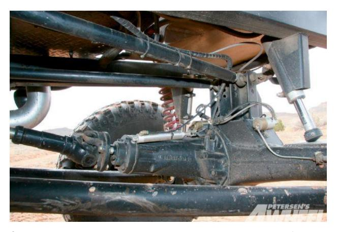
Out back rests a matching 404 Unimog axle that sports an end ratio of 7.56. With the Ford ZF five-speed transmission and four-speed Atlas transfer case, Jon has serious gearing options for a variety of terrain. To control the Unimog's factory cable-actuated lockers, Jon fabricated a set of axle-mounted actuators. In additional to the selectable lockers, he gains even more vehicle control with the electronically controlled cutting brakes on the rear axle.
