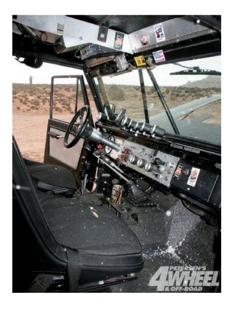
Since much of the protective tubing is cleanly placed outside of the vehicle, the interior is spacious for a two-seat crawler. As owner of JB Custom Fabrication, Jon created most of the interior gadgets by hand and was testing out his new cable shifters for the Atlas transfer case when we caught up with him in Moab.
