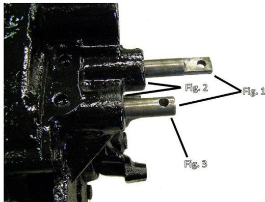
Long: 4-speed applications. Shifter pivot is located approx. 4" from the front of the transfer case.
