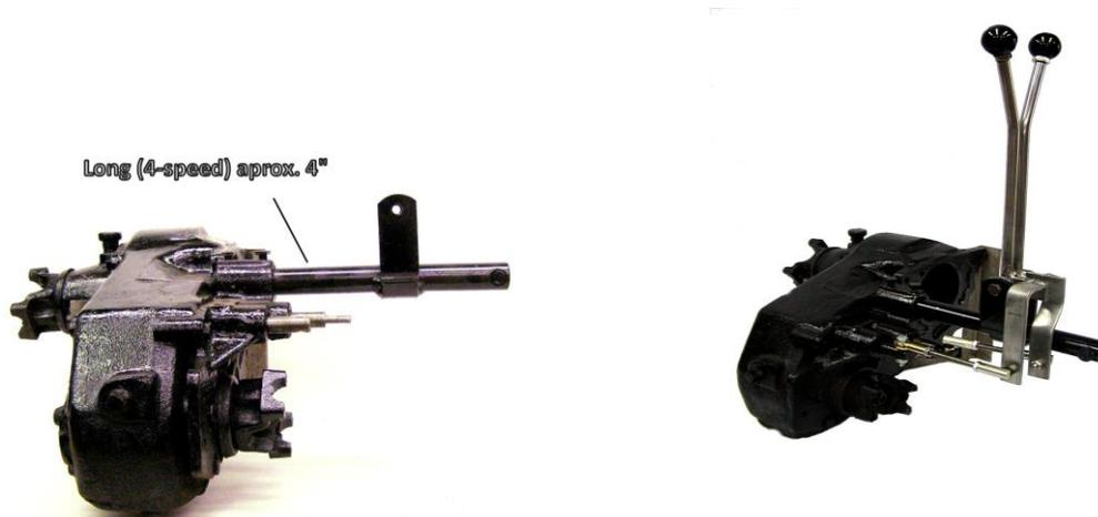
**Short:** 3-speed applications. shifter pivot is located aprox. 1/2" from the front of the transfer case (note: 76'-79' could be clocked 15\* from level from the factory. If the shift-rails are not level with the ground then you have a clocked case that will require our shifter model **D-20CJSC**).
