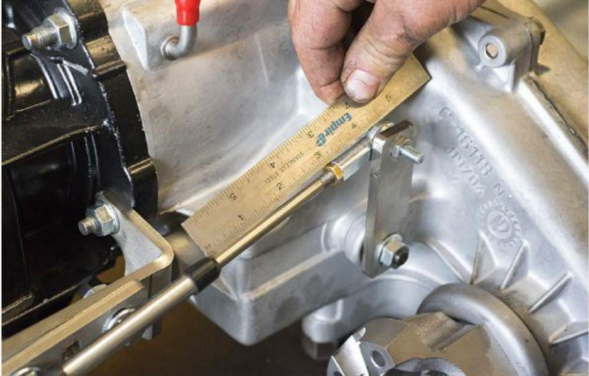
JB's cable is stainless, and uses a stainless steel pivot pin and hardware to attach it to the transfer case. Proper cable adjustment is 3 inches of movement, allowing the transfer case's shift
