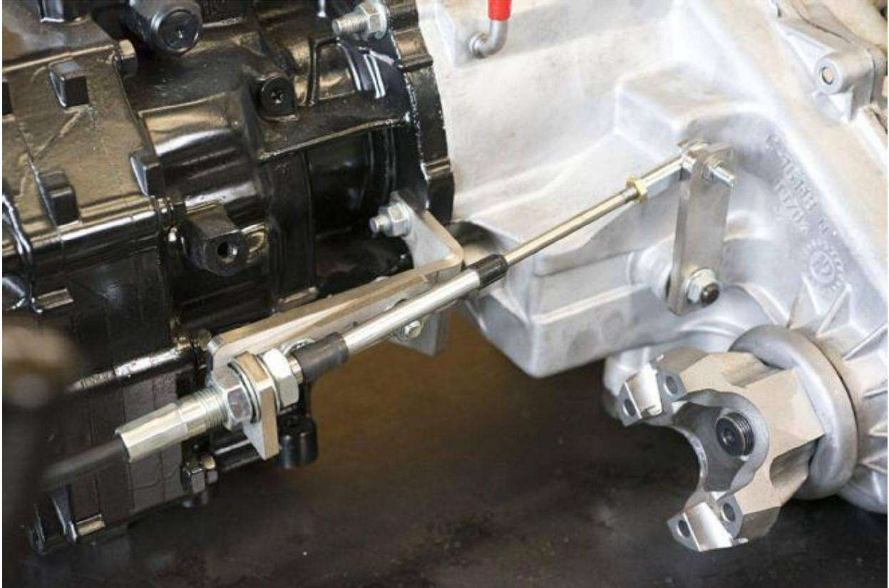
JB Custom Fabrications single-stick transfer case cable-shifter is simple, strong, and well designed, providing smooth and trouble-free T-case range changes.
