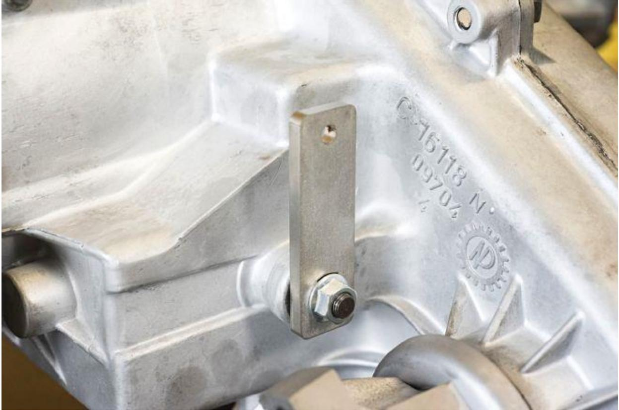
The new shift lever bolts to the transfer case shift arm.
