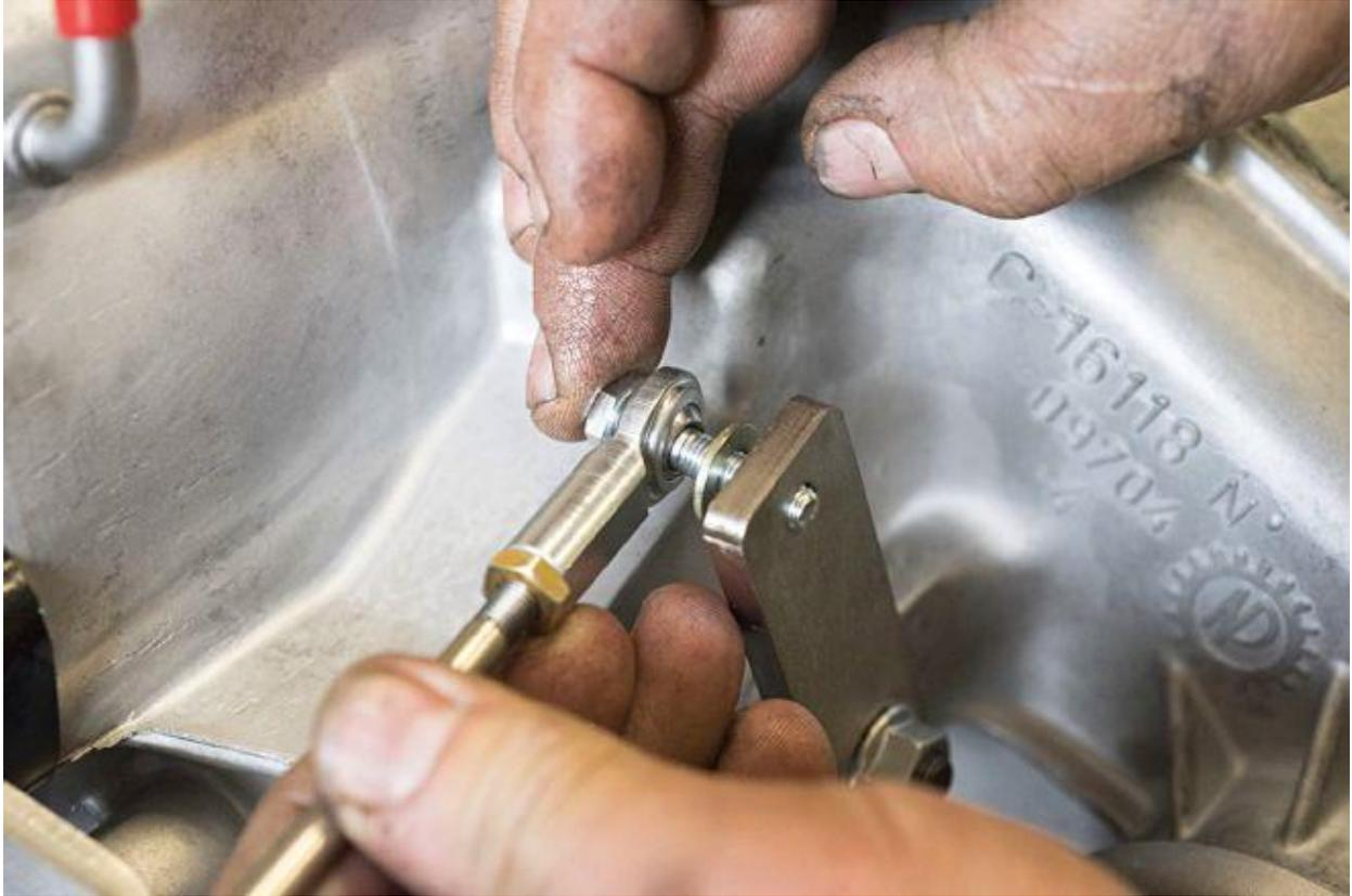
JB's cable is stainless, and uses a stainless steel pivot pin and hardware to attach it to the T-case shift lever.
