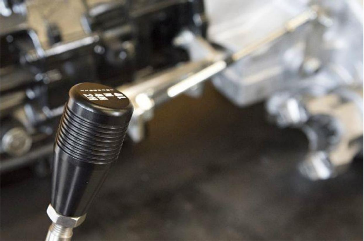
The new shift knob shows the reversed transfer case shift pattern with “4L” forward and “2H” in the rear position.
