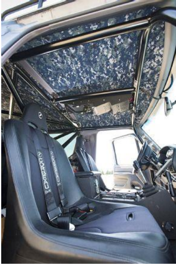
Corbeau seats with safety harnesses are mounted to the interior rollcage assembly.
