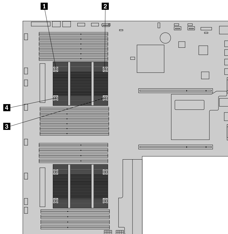
Figure 58. Removing the screws that secure the heat sink
