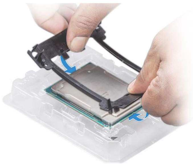
Figure 60. Installing the processor bracket
