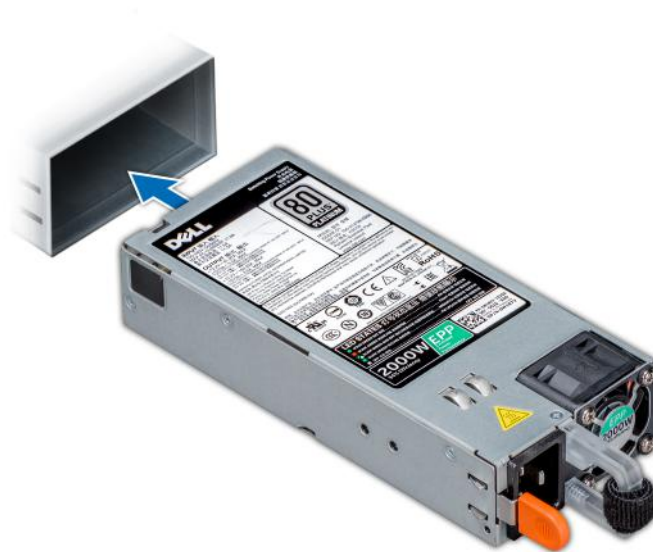
Figure 118. Installing a power supply unit
