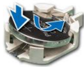
Figure 112. Installing the system battery
