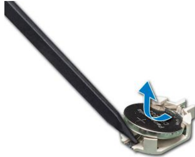
Figure 111. Removing the system battery
