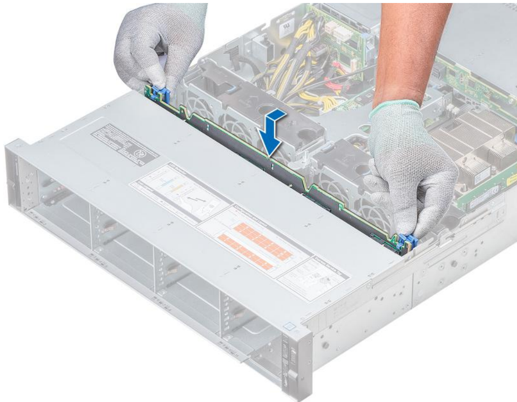
Figure 101. Installing the backplane
