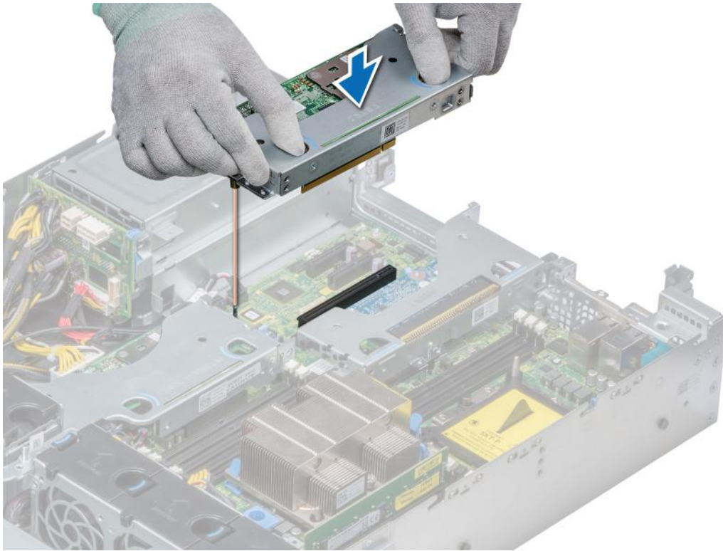
Figure 85. Installing low profile riser left
