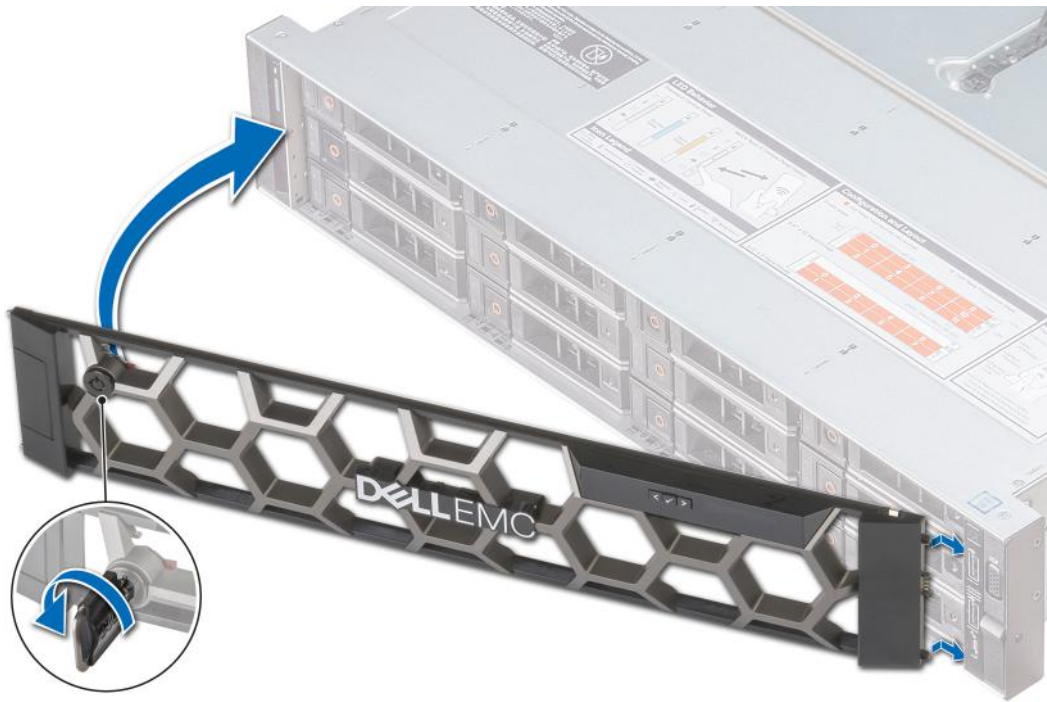
Figure 23. Installing the front bezel with the LCD panel
