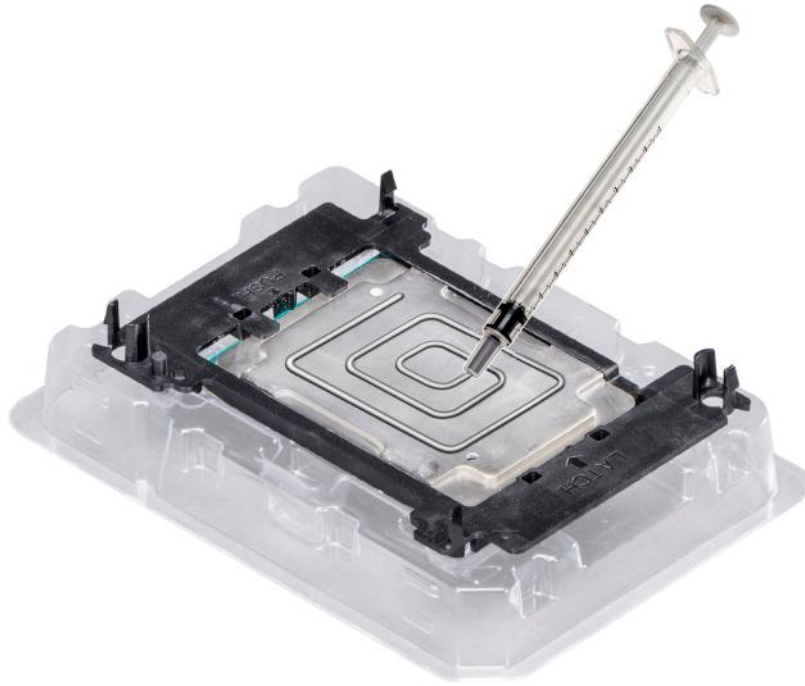
Figure 61. Applying thermal grease on top of the processor
