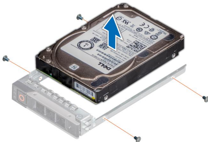
Figure 52. Removing the drive from the drive carrier
