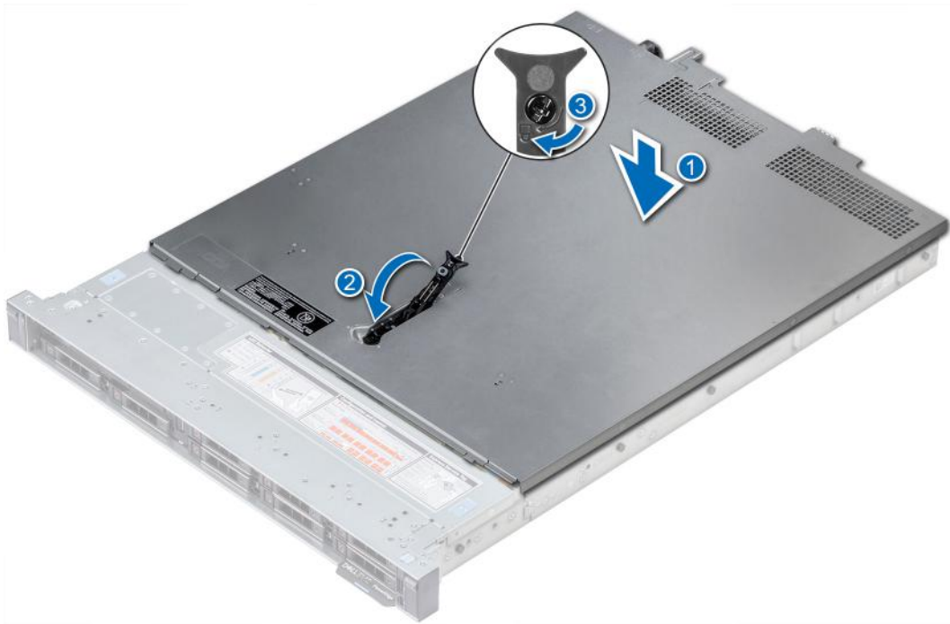
Figure 19. Installing the system cover
