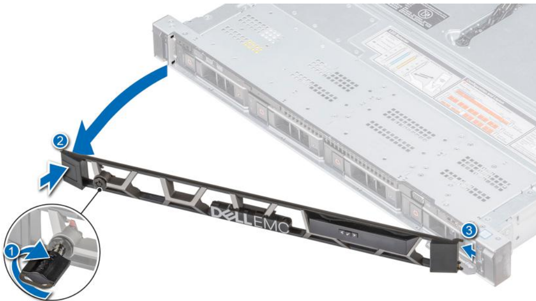
Figure 16. Removing the front bezel with the LCD panel
