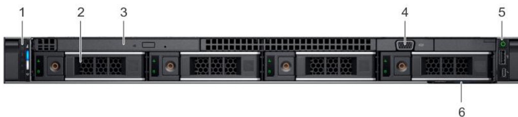
Figure 2. Front view of 4 x 3.5-inch drive system
