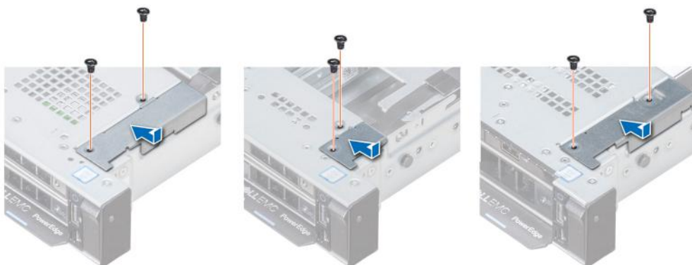
Figure 111. Installing the cable cover
