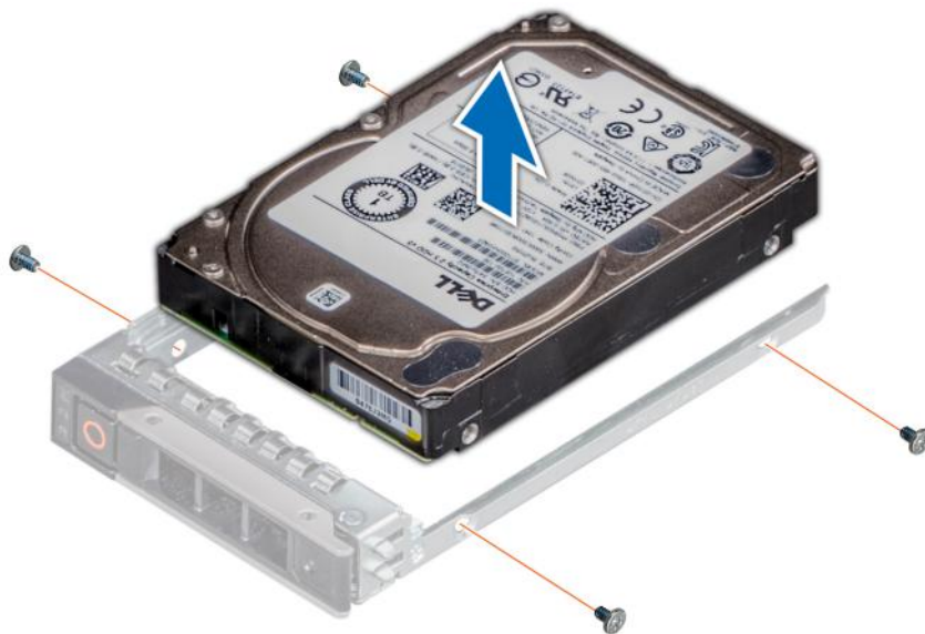
Figure 37. Removing the drive from the drive carrier
