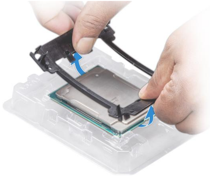
Figure 44. Removing the processor bracket
