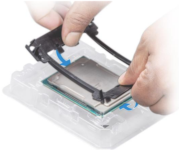
Figure 45. Installing the processor bracket
