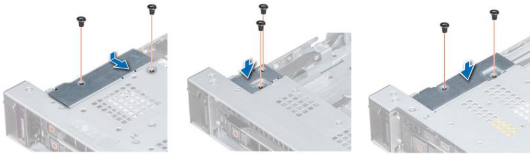
Figure 108. Installing the cable cover
