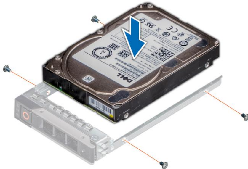
Figure 38. Installing a drive into the drive carrier
