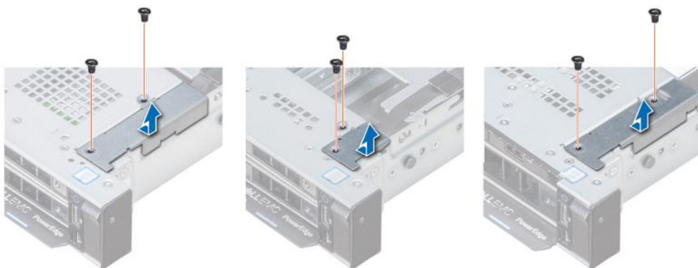
Figure 109. Removing the cable cover
