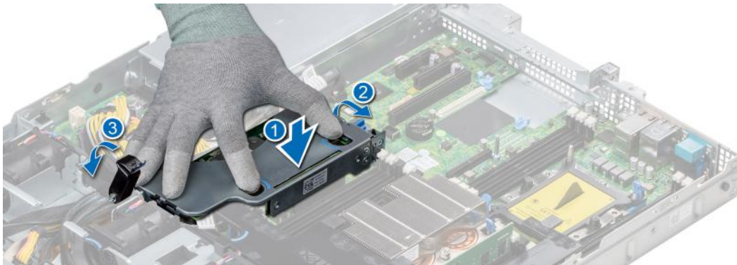
Figure 71. Installing internal PERC riser
