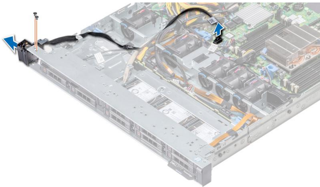
Figure 107. Removing left control panel
