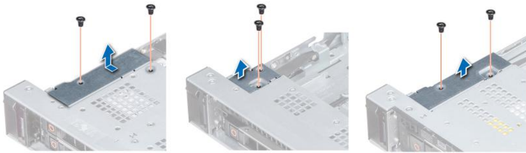
Figure 106. Removing the cable cover
