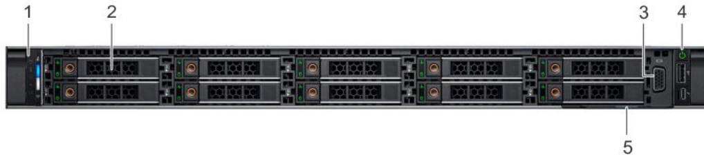
Figure 3. Front view of 10 x 2.5-inch drive system
