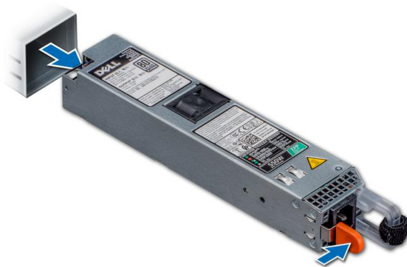
Figure 100. Removing a power supply unit
