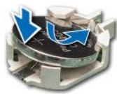
Figure 95. Installing the system battery
