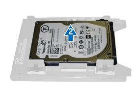
7. If a 3.5-inch hard drive is installed, flex the hard-drive bracket on both sides to loosen the hard drive.
