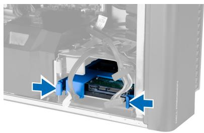
**5.** Slide the hard drive out of the compartment.
