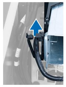
7. Lift the release latch on top of the optical-drive cage.
