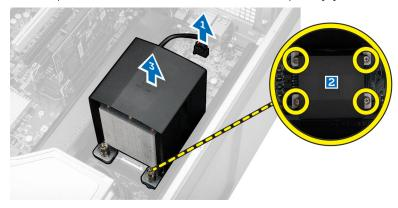
4. Repeat Step 4 to remove the second heatsink module from the computer.
