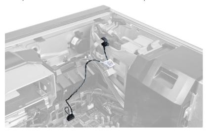
4. Disconnect the HDD thermal sensor cable from the system board.
