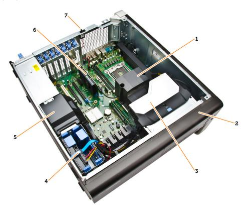
Figure 2. Inside View of T7810 Computer
