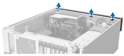
4. Rotate and pull the bezel panel away from the computer to release the hooks on the opposite edge of the bezel from the chassis.
