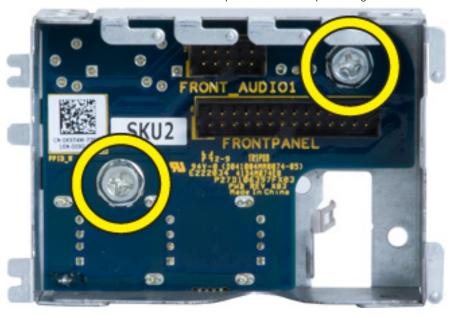
7. Remove the I/O panel from the I/O panel cage.
