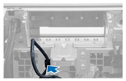
**4.** Remove the screws that secure the drive bay.
