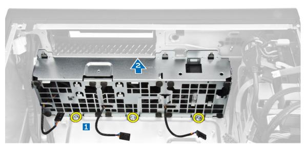
6. Pry away the grommets to remove the system fans from the system-fan assembly.
