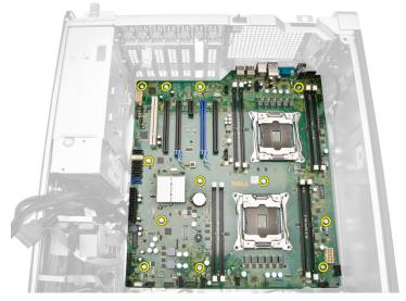
**5.** Slide and lift the system board in an upward direction [1, 2].
