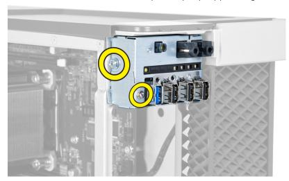
**4.** Remove the I/O panel cage from the chassis.
