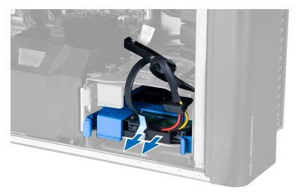
4. Press in on the latches on both sides of the hard-drive bracket.
