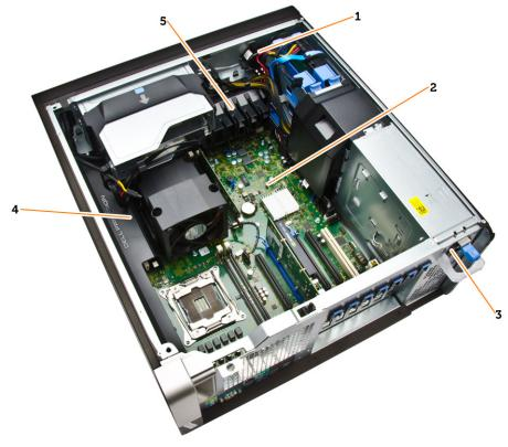
Figure 3. Inside View of T7810 Computer
