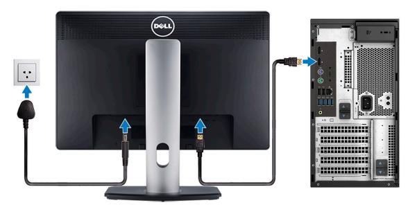
(i) **NOTE:** If you ordered your computer with a discrete graphics card, the HDMI and the display ports on the back panel of your computer are covered. Connect the display to the discrete graphics card.
