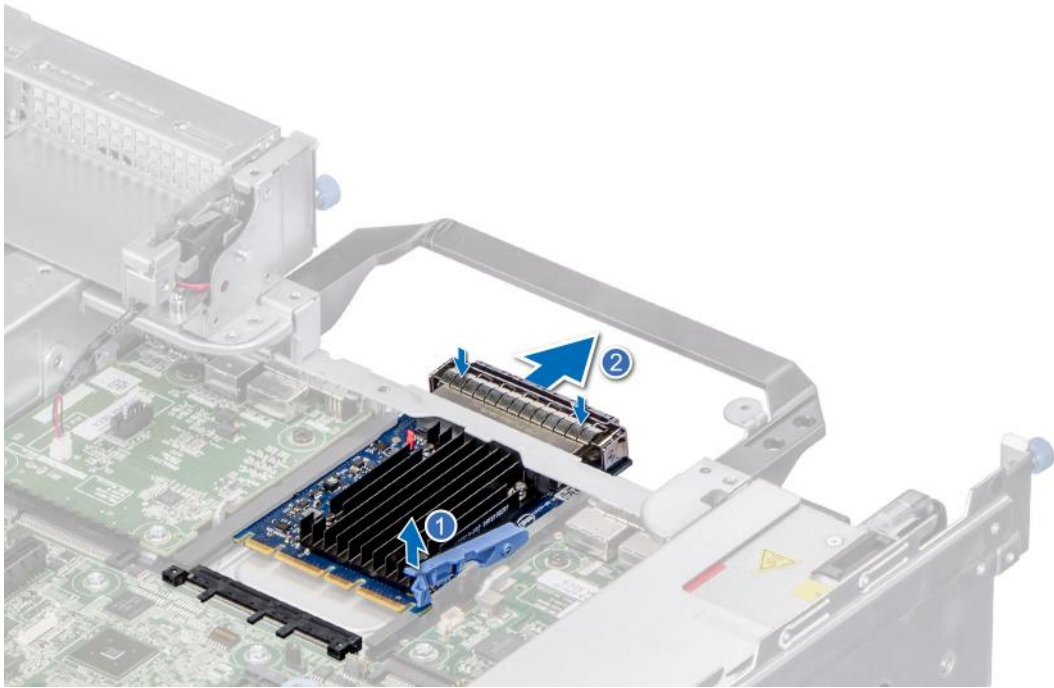
Figure 140. Removing the OCP card
