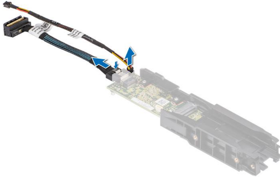
Figure 101. Removing the BOSS power cable and BOSS signal cable from the BOSS S2 controller card module
