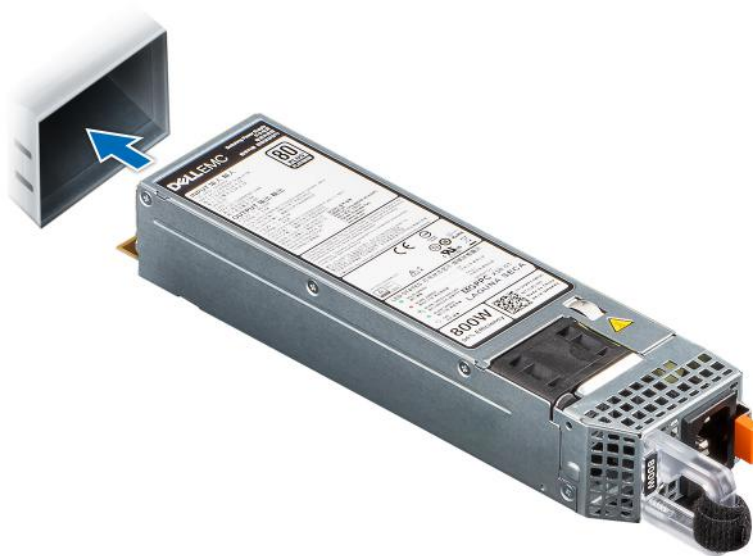
Figure 145. Installing a power supply unit
