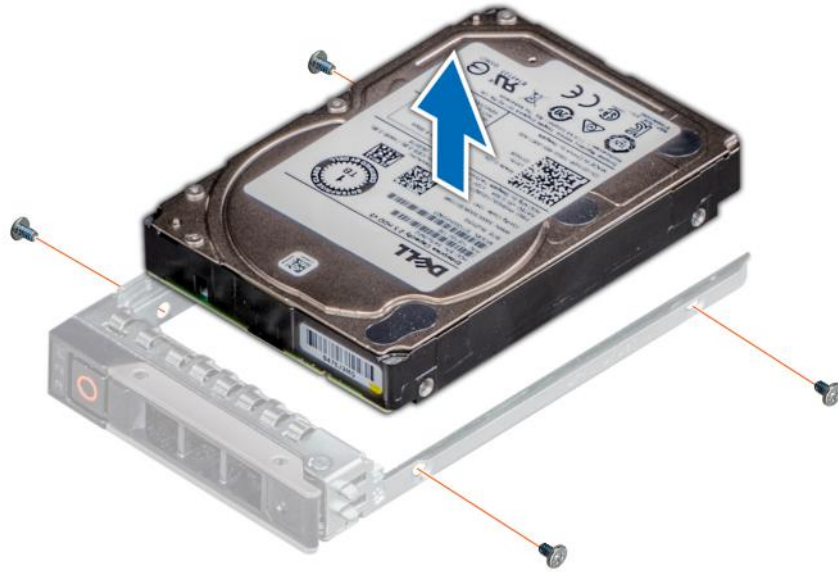
Figure 44. Removing the drive from the drive carrier
