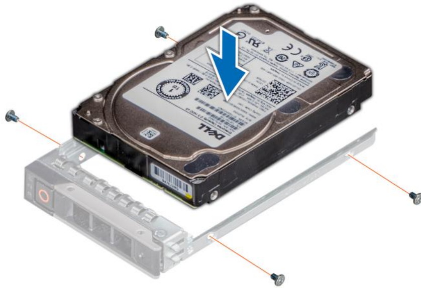
Figure 45. Installing a drive into the drive carrier
