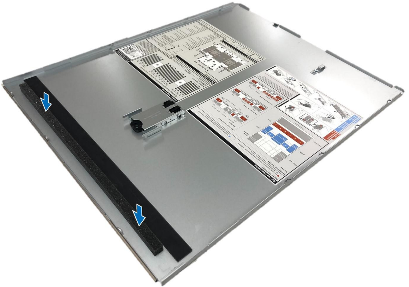
Figure 155. Installing Mylar foam on the system cover
