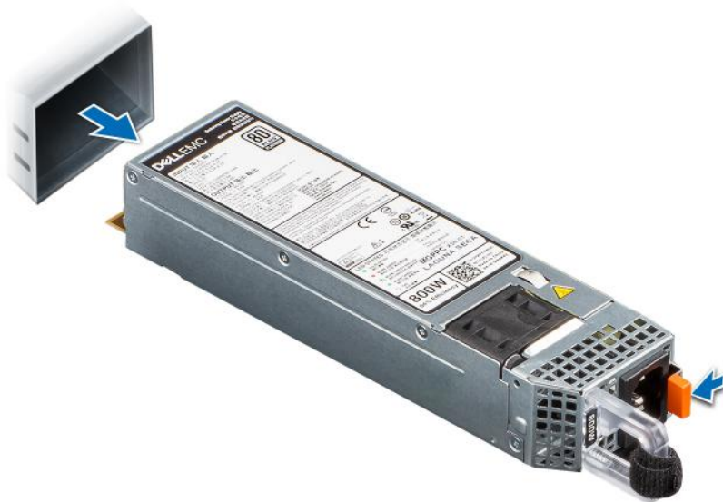
Figure 144. Removing a power supply unit
