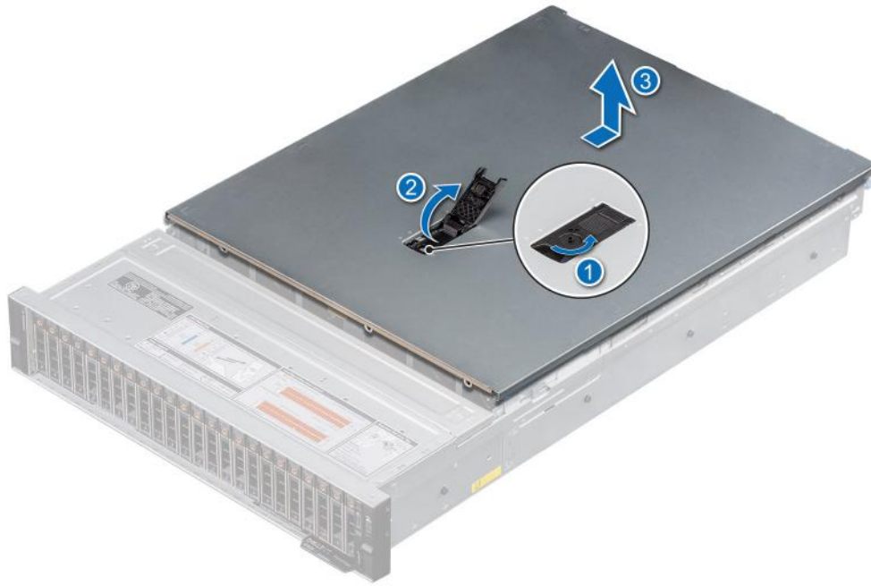
Figure 20. Removing the system cover
