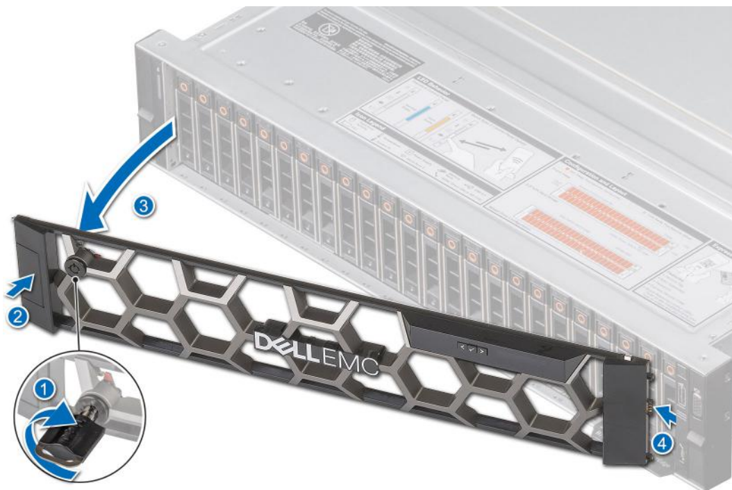
Figure 18. Removing the front bezel
