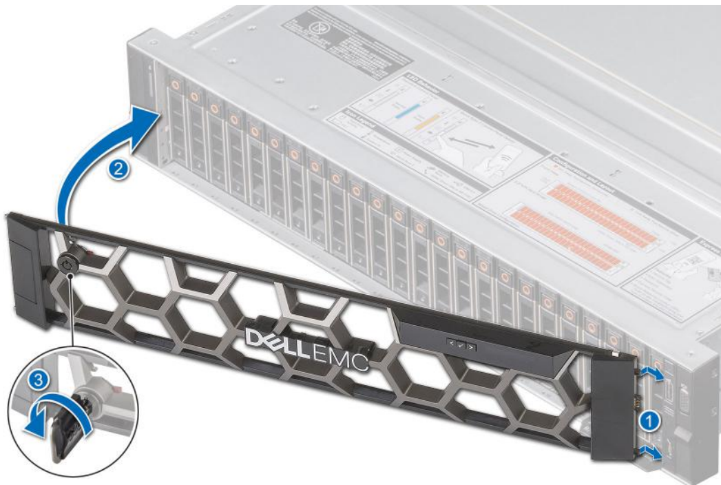
Figure 19. Installing the front bezel
