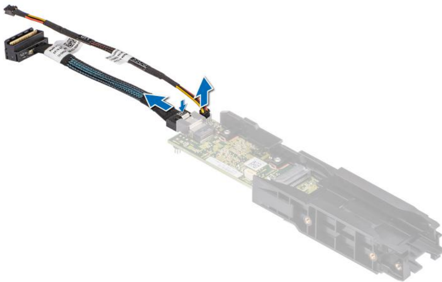
Figure 88. Removing the BOSS power cable and BOSS signal cable from the BOSS S2 controller card module
