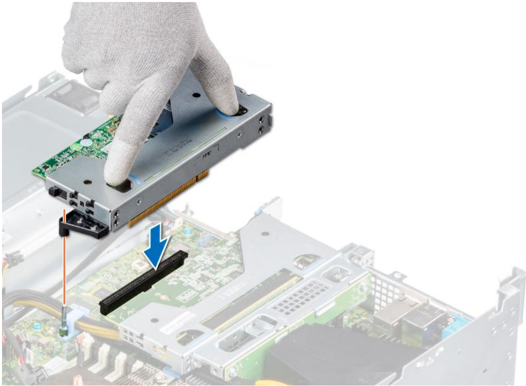
Figure 69. Installing the riser 2
