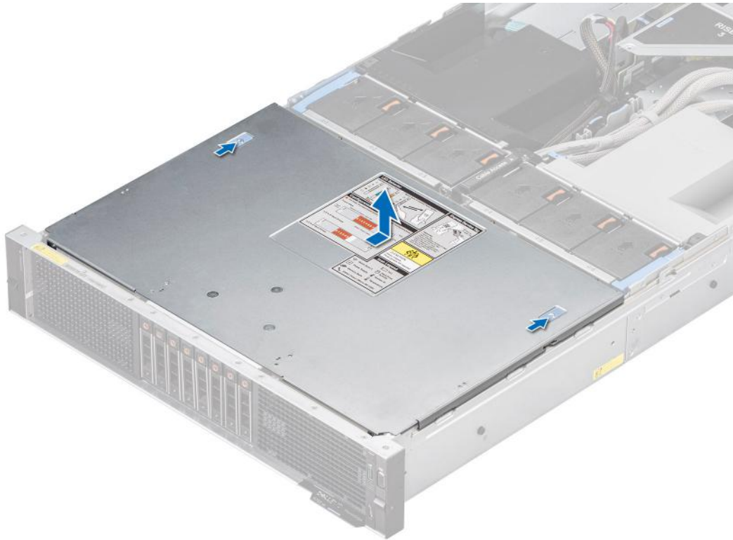
Figure 25. Removing the drive backplane cover
