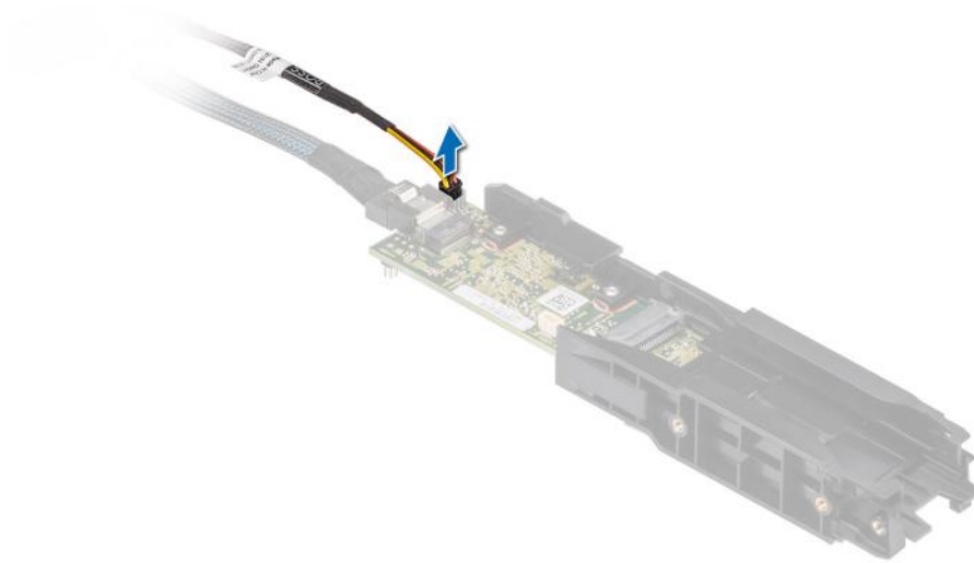
Figure 81. Disconnecting the BOSS S2 power cable
