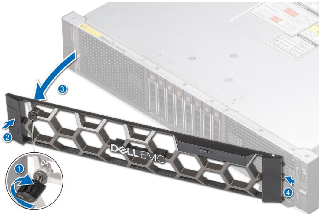
Figure 21. Removing the front bezel
