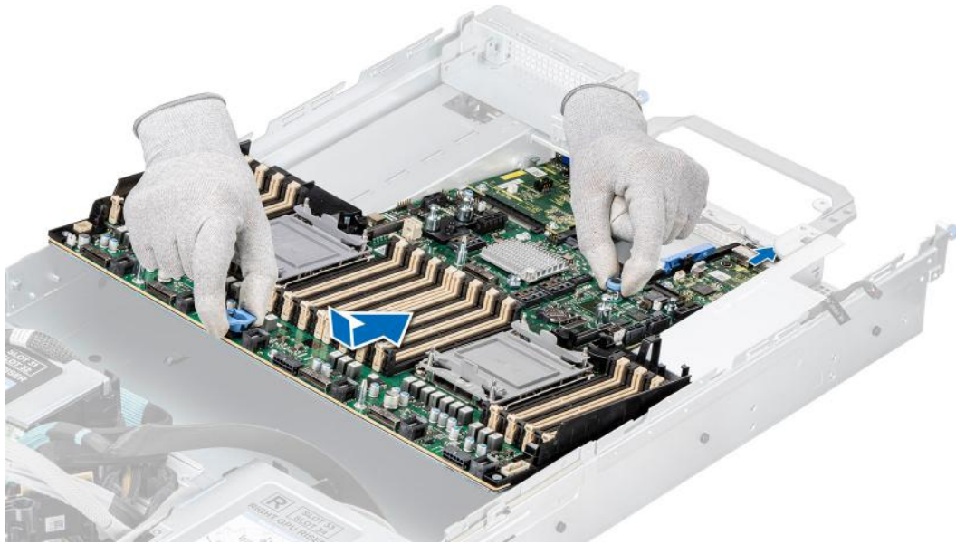
Figure 169. Installing the system board
