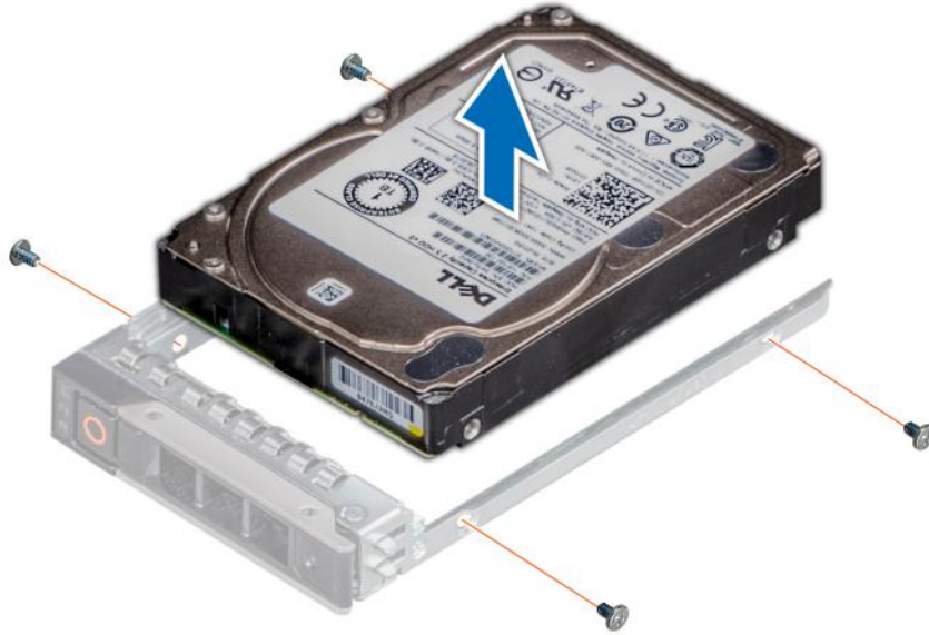
Figure 42. Removing the drive from the drive carrier
