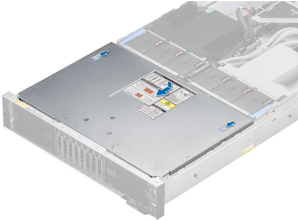
Figure 26. Installing the drive backplane cover
