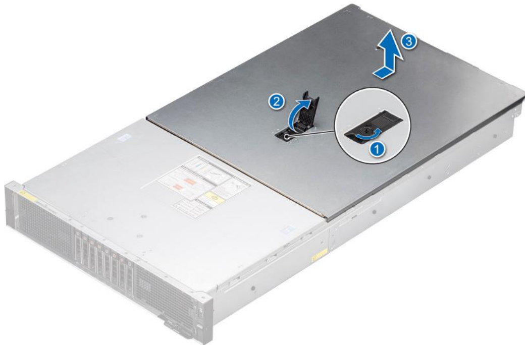
Figure 23. Removing the system cover
