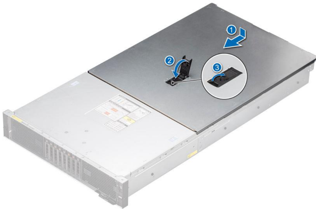
Figure 24. Installing the system cover
