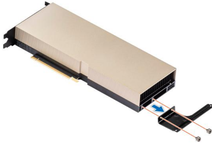
Figure 102. Removing the standard bracket with two screws
