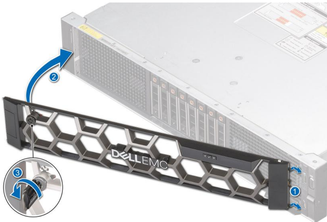
Figure 22. Installing the front bezel
