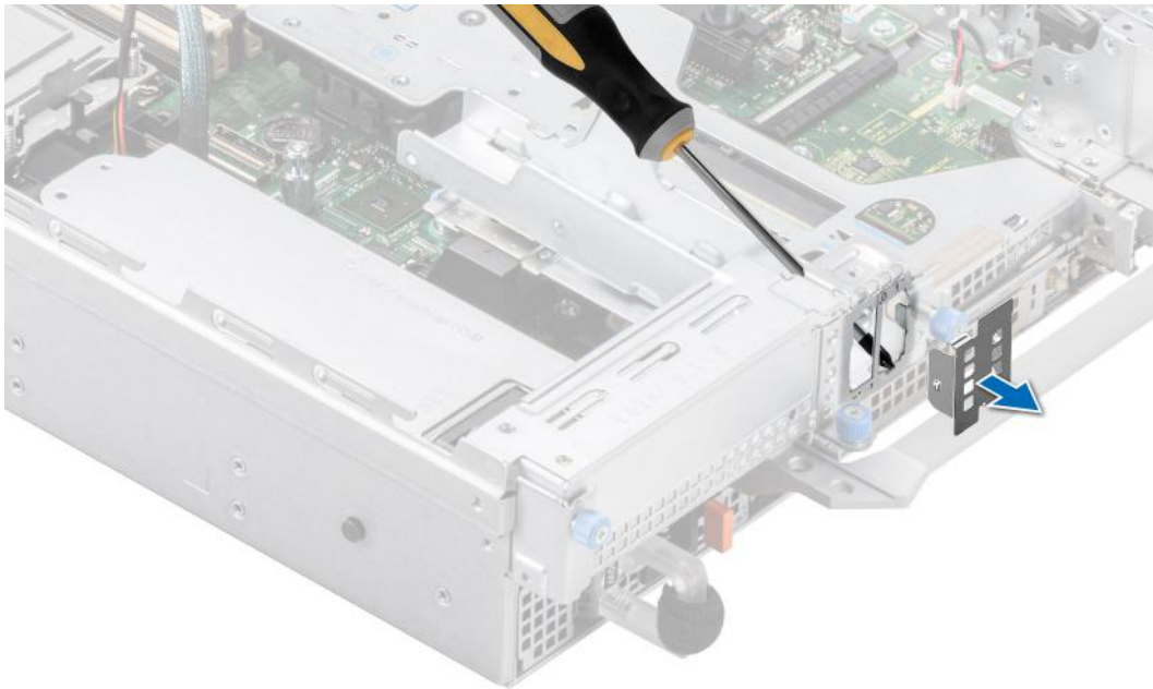
Figure 178. Removing the BOSS S2 module blank
