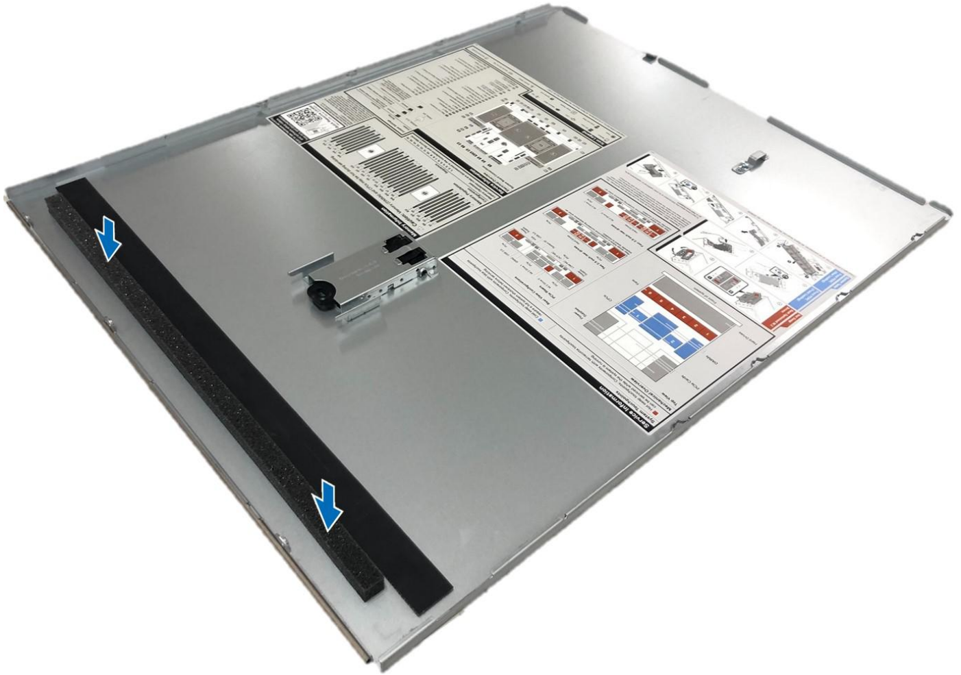
Figure 224. Installing Mylar foam on the system cover
