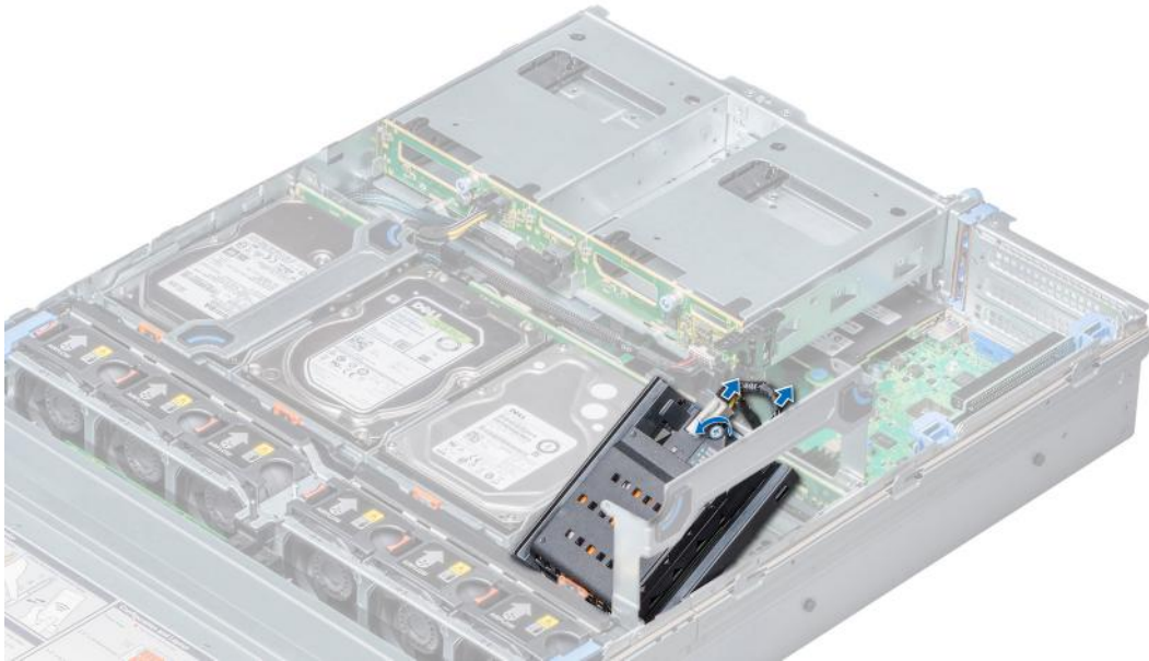
Figure 41. Removing NVDIMM-N battery from mid drive tray
