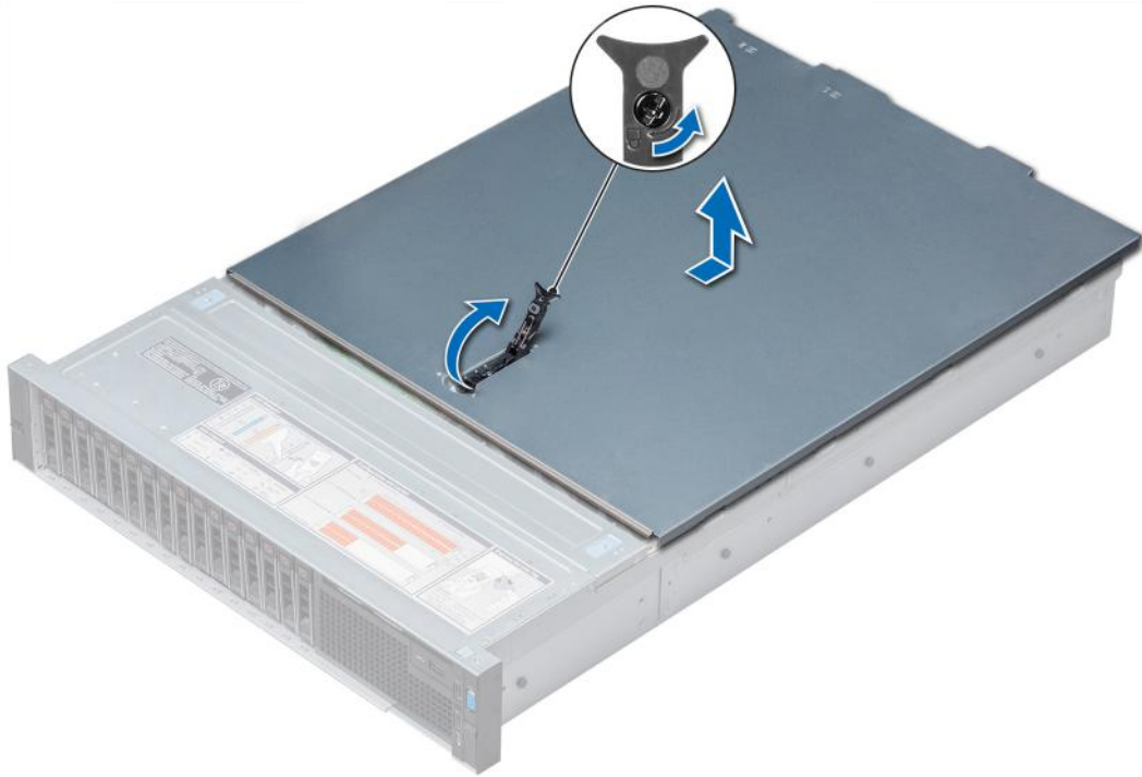
Figure 25. Removing the system cover
