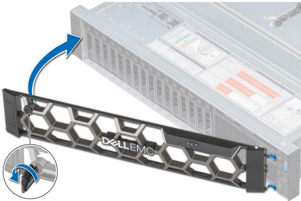
Figure 24. Installing the optional front bezel with the LCD panel
