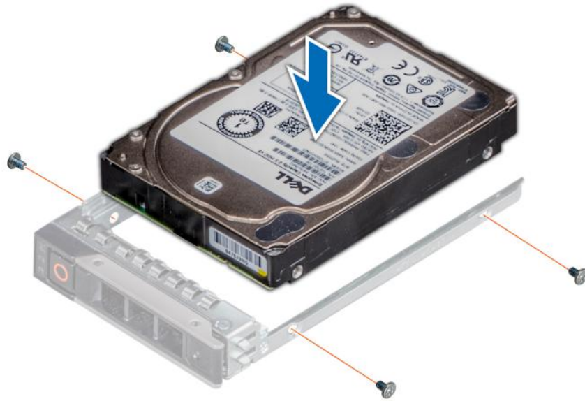
Figure 64. Installing a drive into the drive carrier
