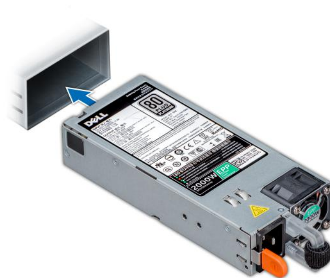
Figure 166. Installing a power supply unit
