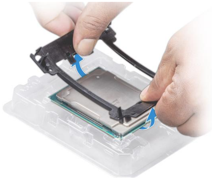
Figure 74. Removing the processor bracket
