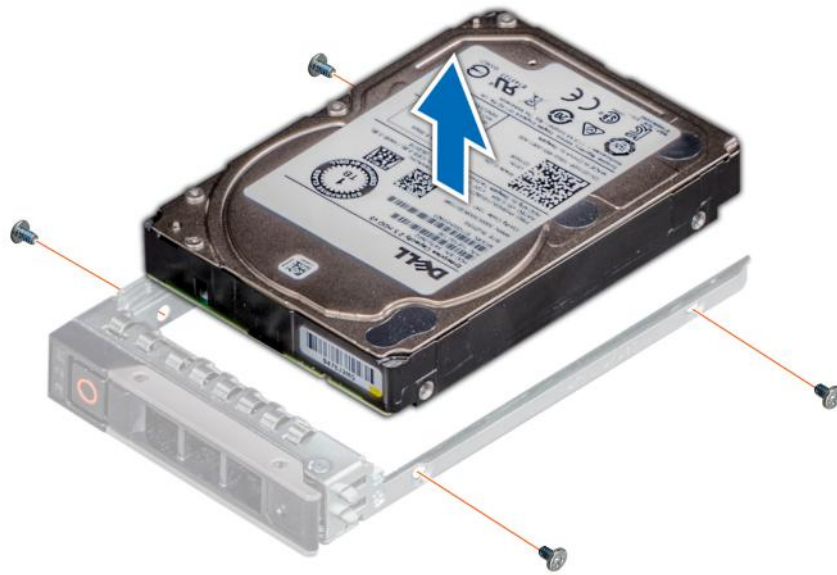
Figure 63. Removing the drive from the drive carrier
