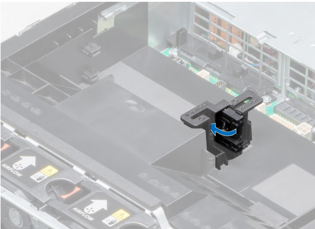
Figure 81. Closing the PCIe card holder latch
