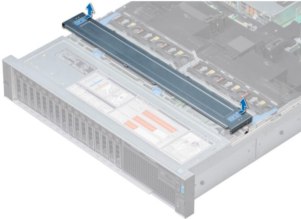
Figure 27. Removing backplane cover
