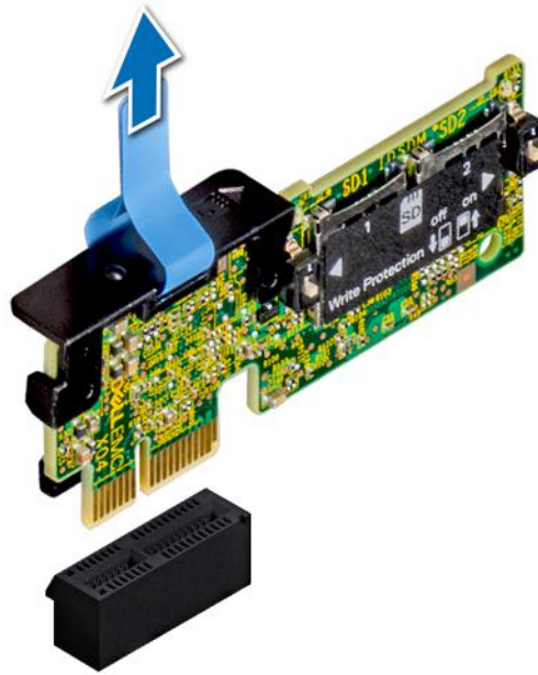
Figure 116. Removing the optional IDSDM/vFlash module
