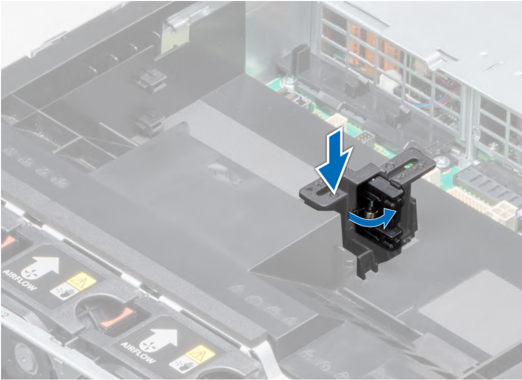
Figure 80. Opening the PCIe card holder latch
