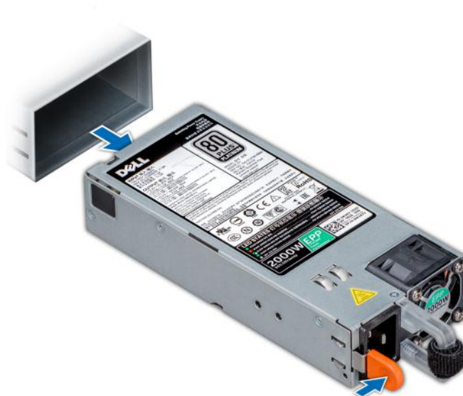
Figure 165. Removing a power supply unit
