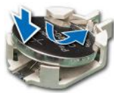
Figure 162. Installing the system battery
