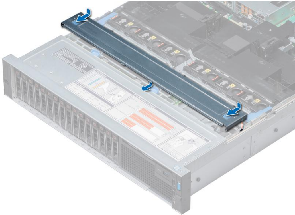
Figure 28. Installing the backplane cover
