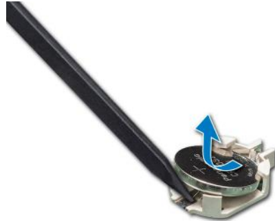
Figure 161. Removing the system battery
