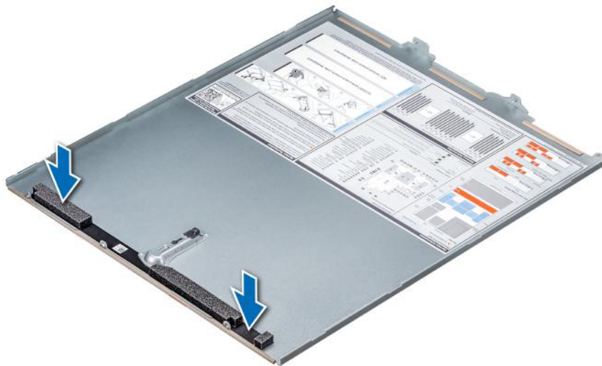
Figure 97. Installing mylar foam on the system cover
