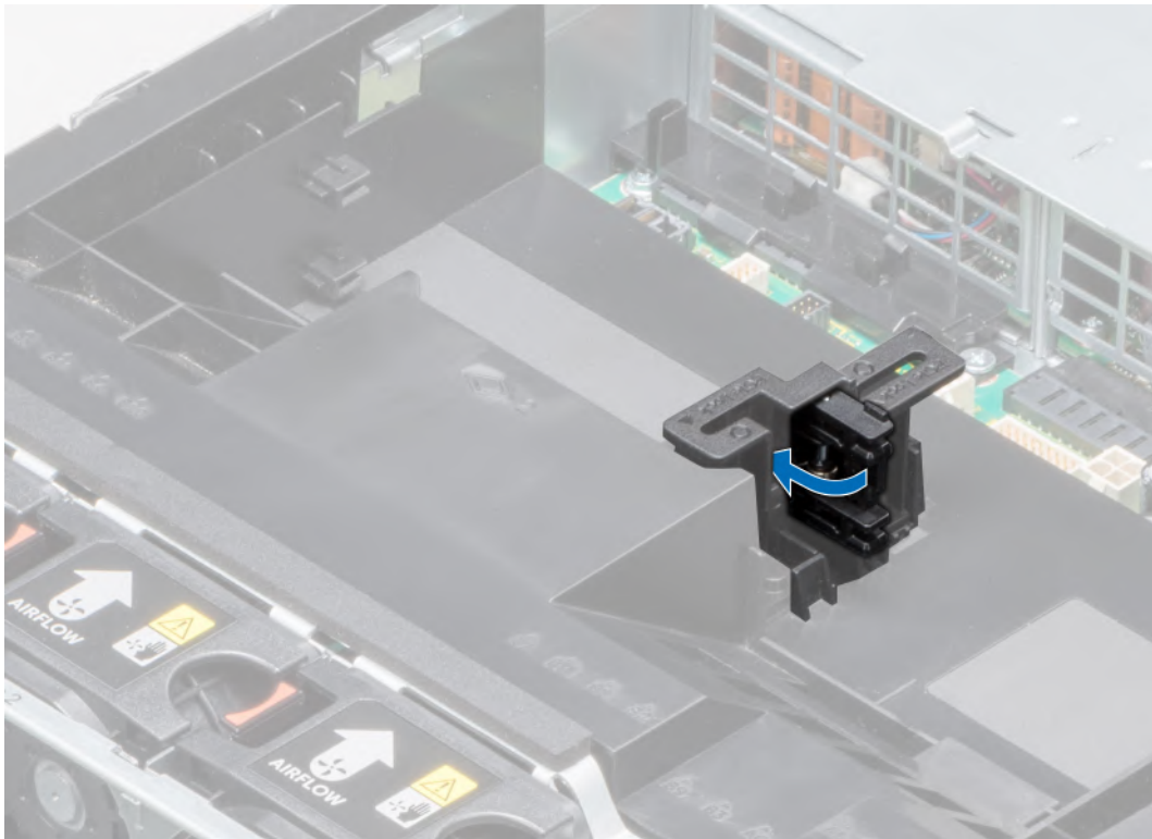
Figure 65. Closing the PCIe card holder latch
