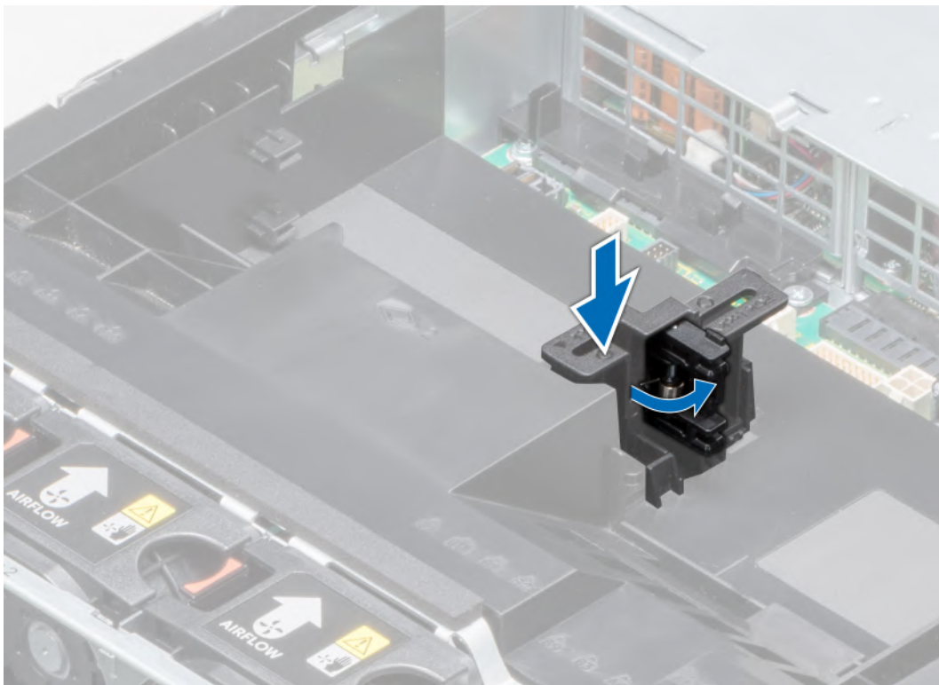
Figure 64. Opening the PCIe card holder latch
