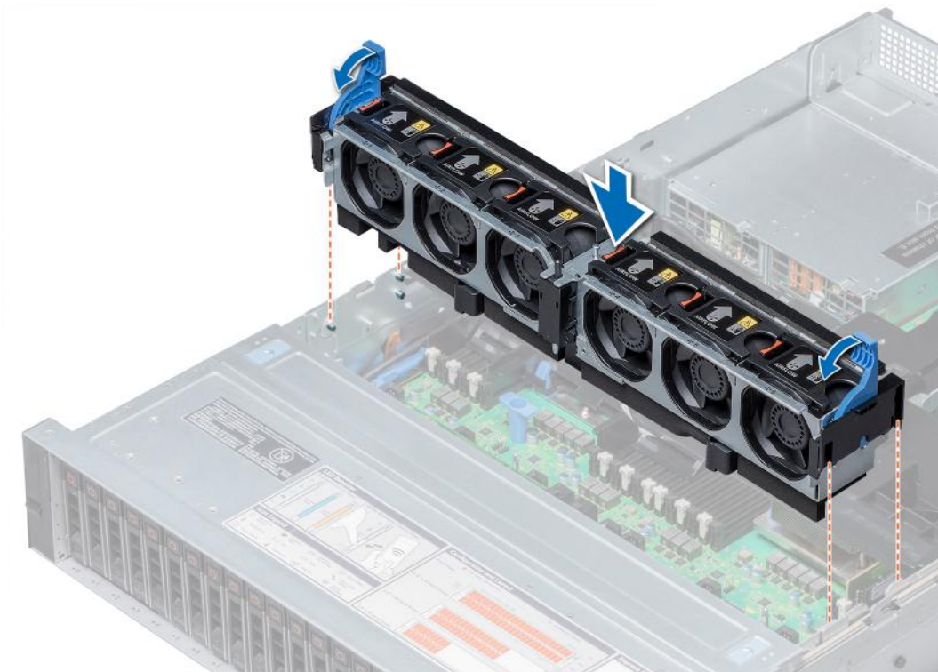
Figure 34. Installing the cooling fan assembly
