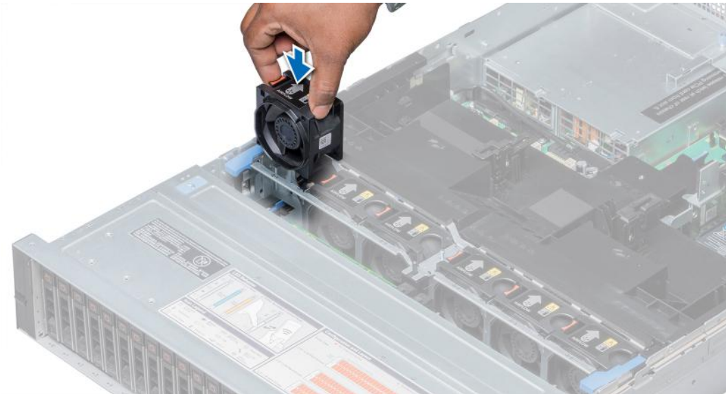
Figure 36. Installing cooling fan
