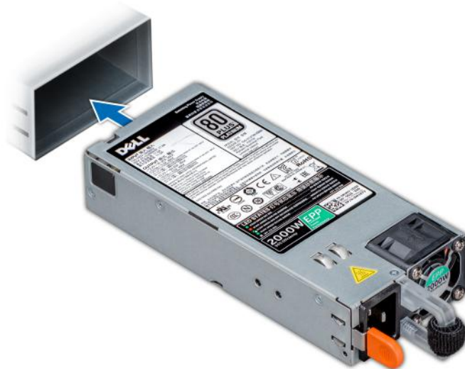
Figure 129. Installing a power supply unit
