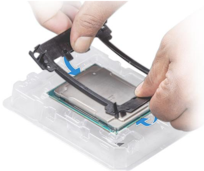
Figure 60. Installing the processor bracket
