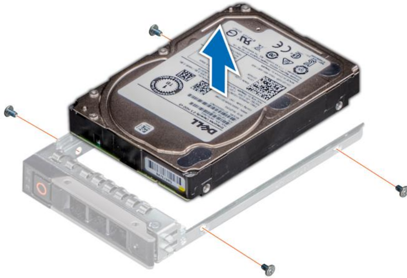
Figure 53. Removing the drive from the drive carrier
