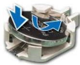
Figure 121. Installing the system battery
