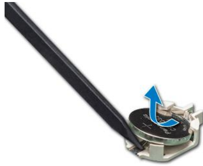
Figure 120. Removing the system battery
