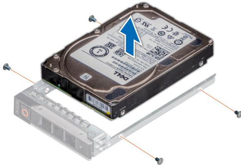
Figure 40. Removing the drive from the drive carrier
