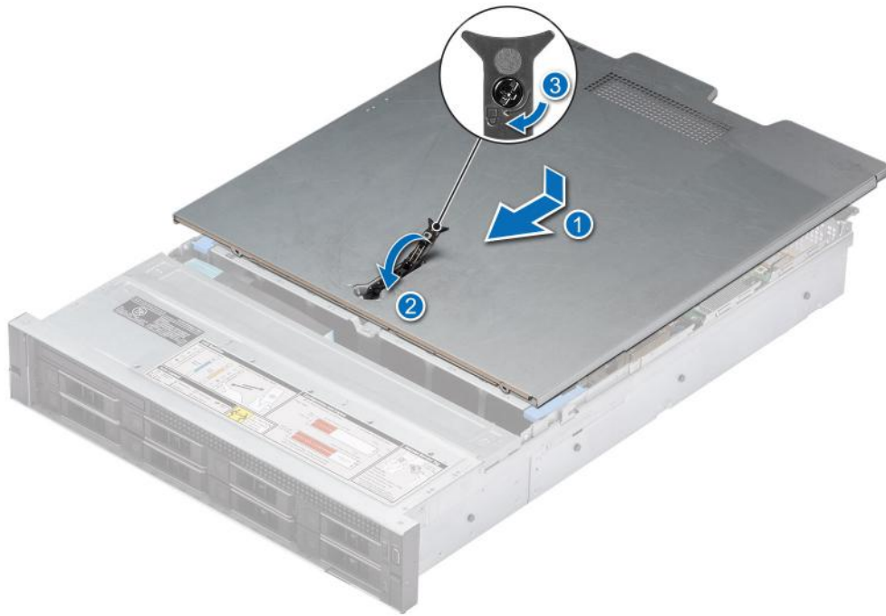
Figure 21. Installing the system cover
