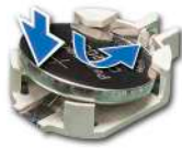
Figure 101. Installing the system battery
