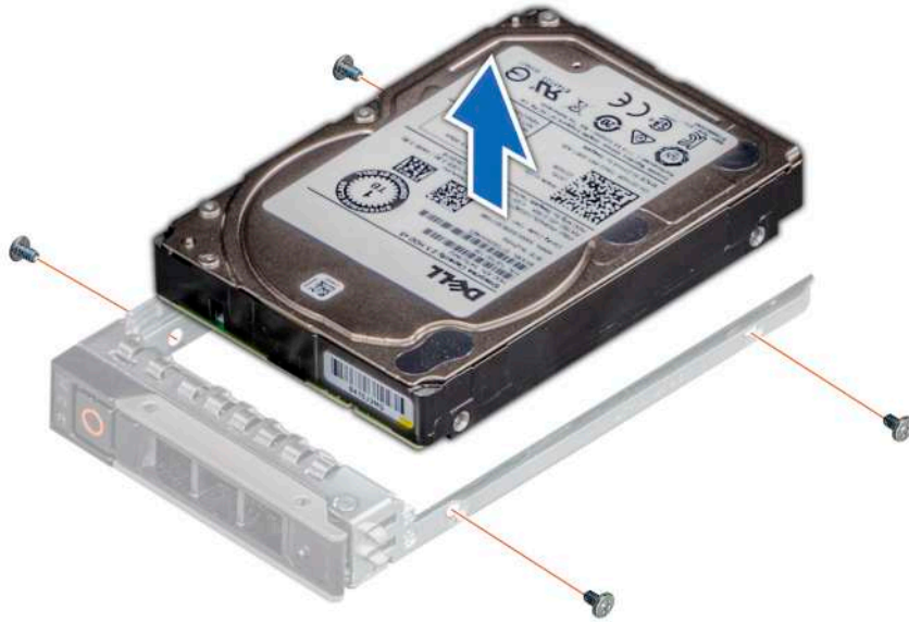
Figure 42. Removing the drive from the drive carrier
