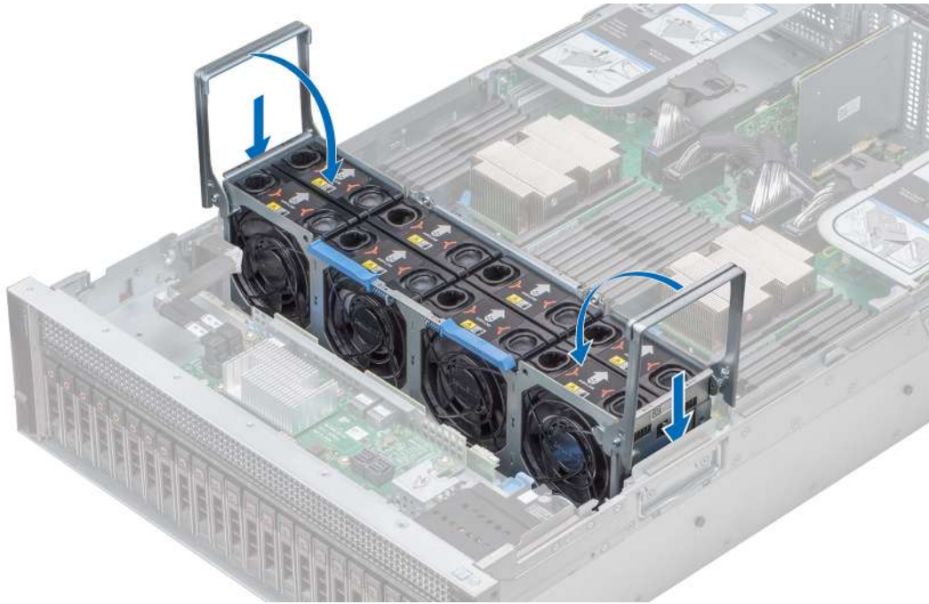
Figure 33. Installing the fan cage
