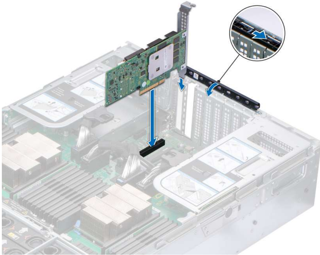
Figure 88. Installing the storage controller card
