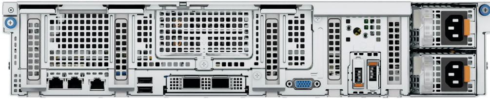
Figure 6. 3 x PCIe Low-Profile Slots with 1 CPU
