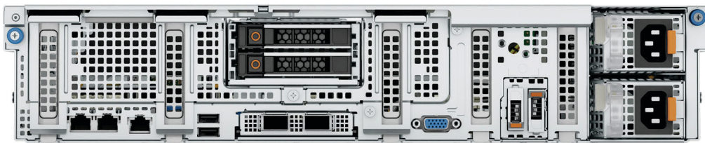
Figure 7. 5 x PCIe Low-Profile Slots + 2 x 2.5-inch NVMe Drives
