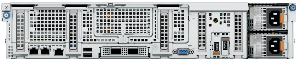
Figure 5. 5 x PCIe Low-Profile Slots
