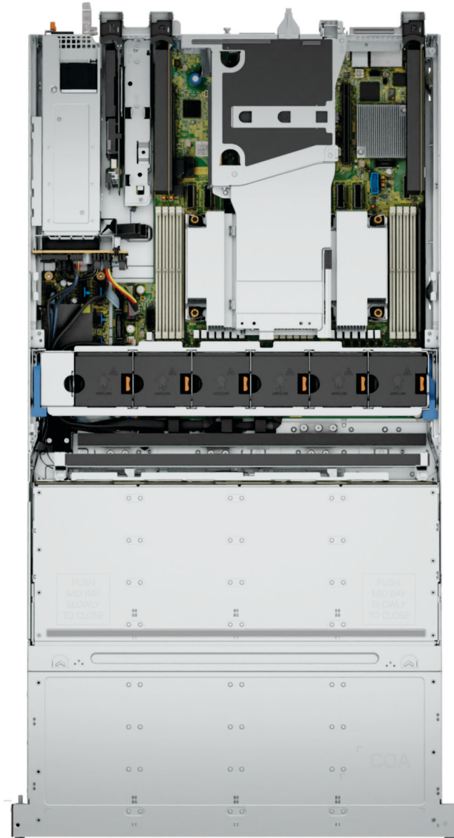
Figure 17. 3 x PCIe Low-Profile Slots + 2 x PCIe FH/FL Slots
