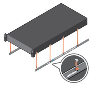
Figure 45. Attach the inner rails to the system
