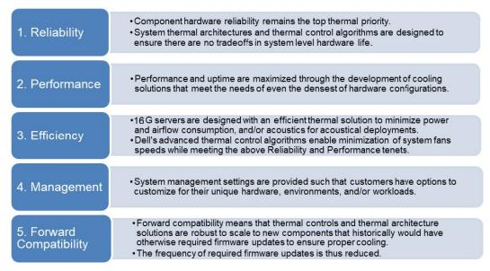
Figure 32. Thermal design characteristics
