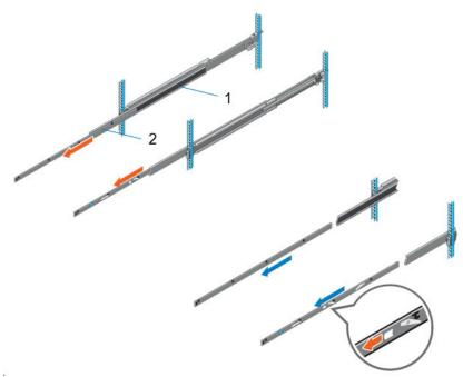
Figure 44. Pull out the intermediate rail
