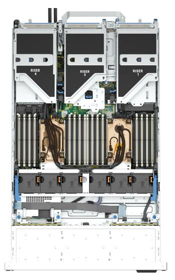
Figure 11. Inside the system with processor liquid cooling module
