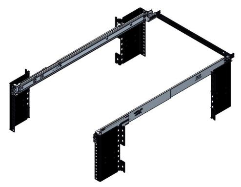
Figure 34. Sliding rails with optional SRB
