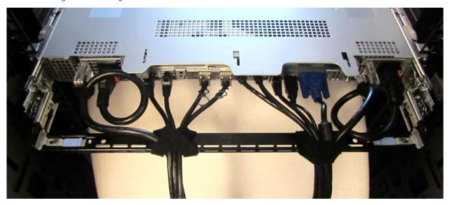
Figure 40. Cabled strain relief bar
