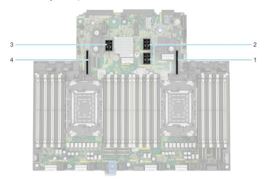
Figure 13. Riser connector location on system board
