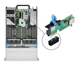
Figure 58. Internal USB Port
