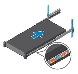
Figure 47. Slide system into the rack
