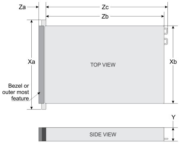
Figure 1. System dimensions of PowerEdge R7425 system
