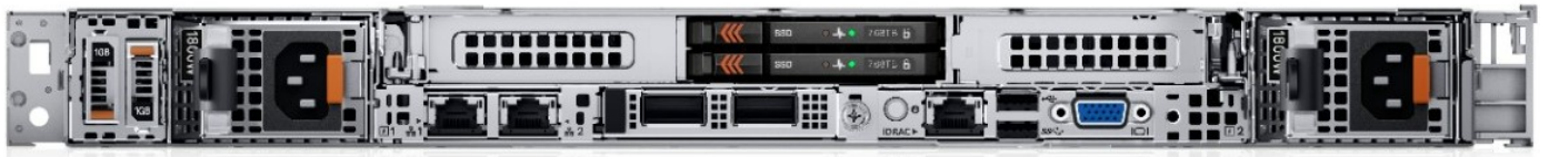
Figure 8. Rear view of the system with 2 x E3.S rear drive system
