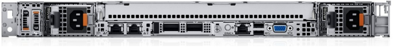
Figure 6. Rear view of the system with no risers
