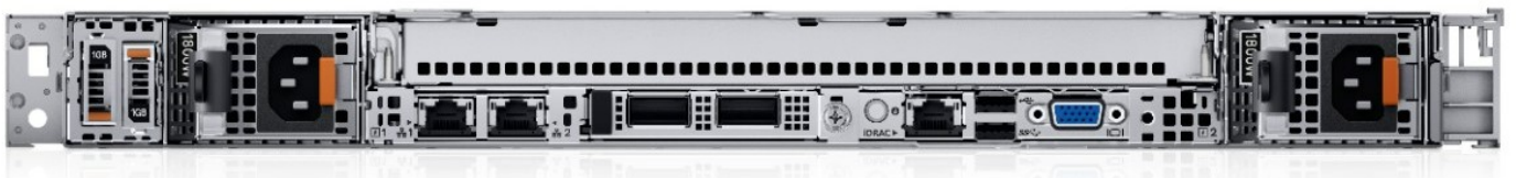
Figure 4. Rear view of the system with no risers
