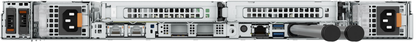
Figure 6. Rear view of the system with Direct Liquid Cooling module
