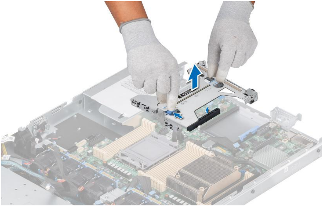
Figure 72. Removing the Riser 2c
