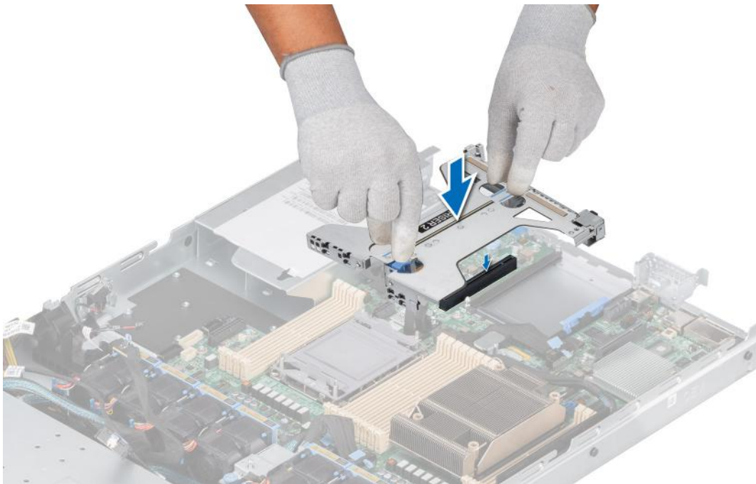
Figure 76. Installing the Riser 2c
