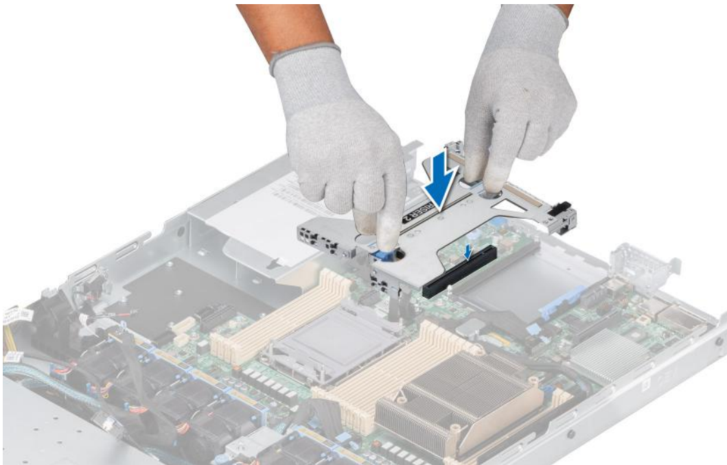
Figure 74. Installing the Riser 2a
