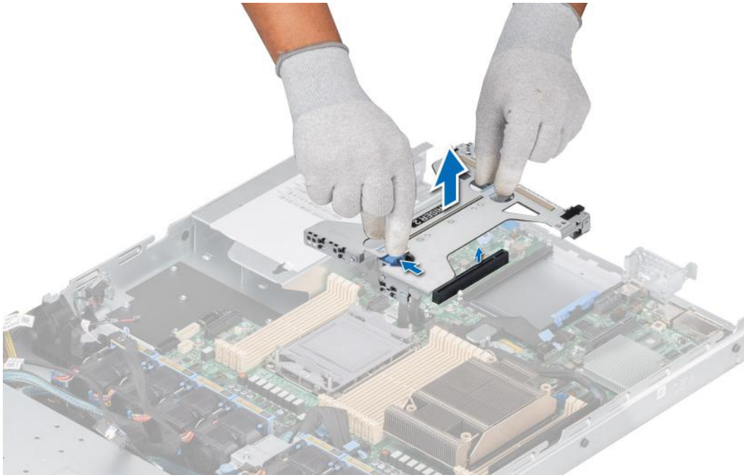
Figure 70. Removing the Riser 2a
