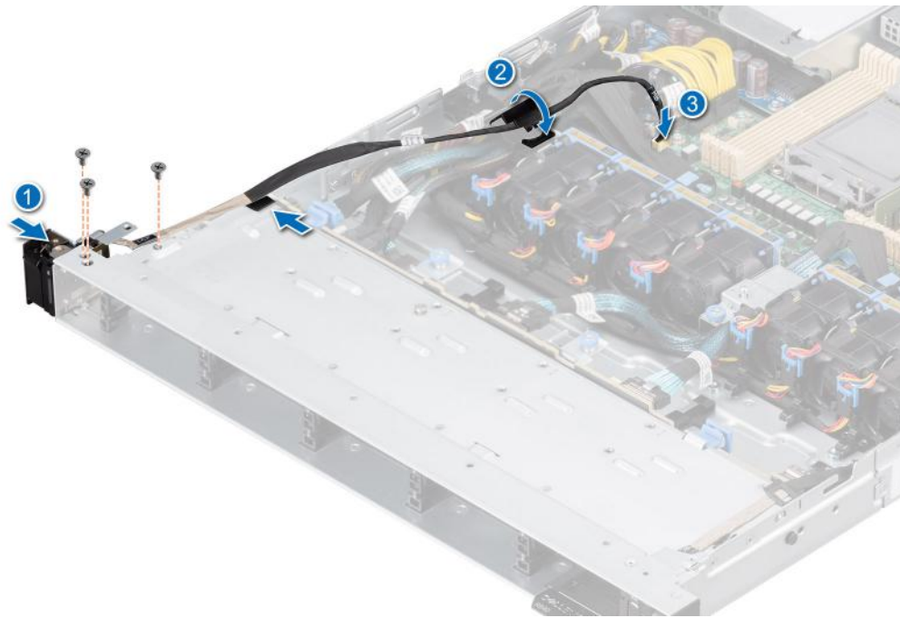
Figure 129. Installing the left control panel
