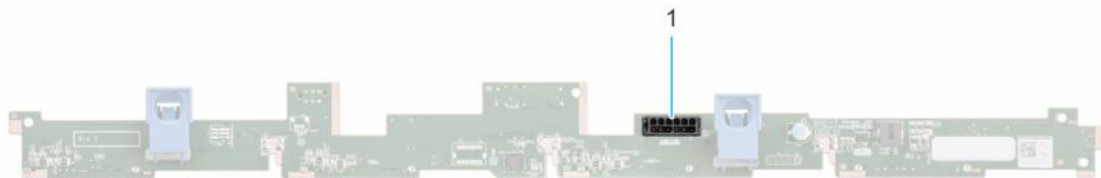
Figure 32. 4 x 3.5-inch drive backplane
