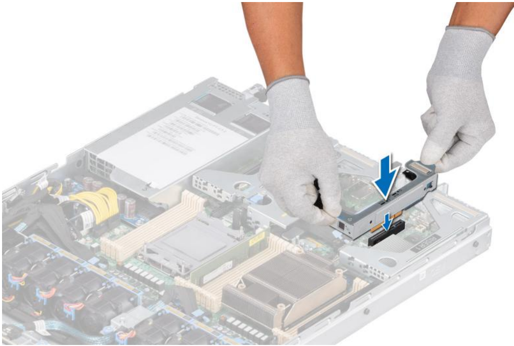
Figure 102. Installing the M.2 BOSS riser
