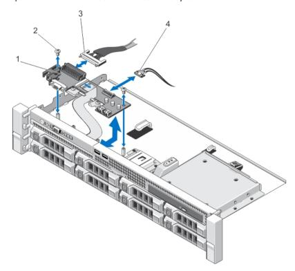
Figure 54. Removing and Installing the Control-Panel Board
