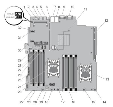
Figure 56. System Board Connectors and Jumpers
