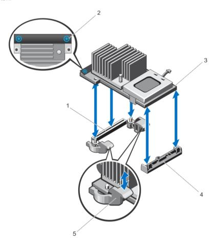
Figure 37. Removing and Installing the Integrated Storage Controller
