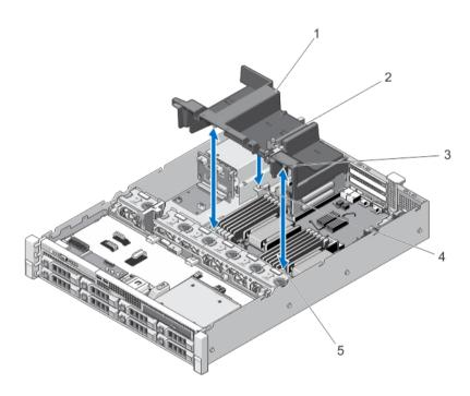
Figure 15. Removing and Installing the Cooling Shroud
