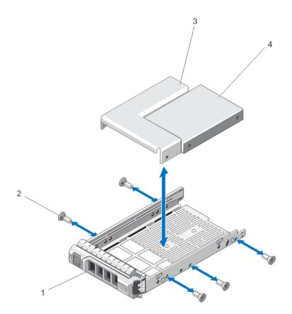
Figure 26. Removing and Installing a Hard-Drive Adapter Into a 3.5 Inch Hard-Drive Carrier
