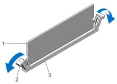
Figure 17. Ejecting The Memory Module
