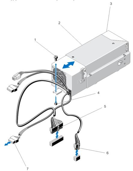
Figure 48. Removing and Installing a Non-Redundant Power Supply
