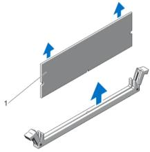
Figure 18. Removing The Memory Module
