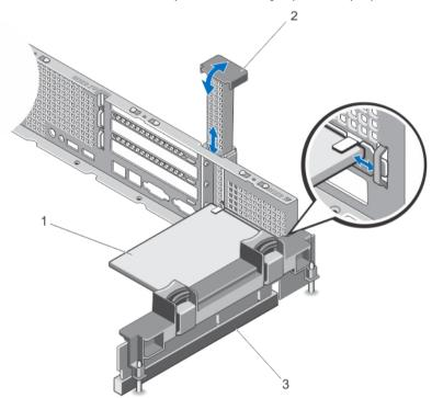
Figure 30. Removing and Installing the Expansion Card from Expansion-Card Riser 1
