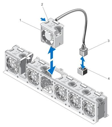
Figure 28. Removing and Installing a Cooling Fan
