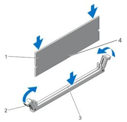
Figure 19. Installing The Memory Module
