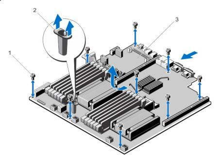
Figure 55. Removing and Installing the System Board
