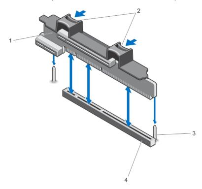
Figure 32. Removing and Installing the Expansion-Card Riser 1
