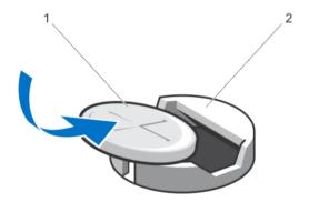
Figure 50. Replacing the System Battery
