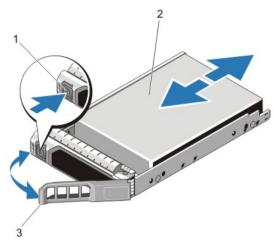
Figure 23. Removing and Installing a Hot-Swap Hard Drive
