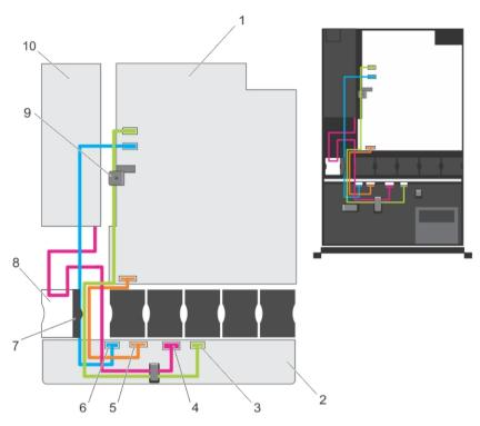
Figure 53. Cabling Diagram of the Hard-Drive Backplane for a Non-Redundant PSU System
