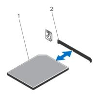
Figure 35. Removing and Installing the SD vFlash Card
