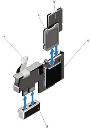
Figure 36. Removing and Installing the Internal Dual SD Module
