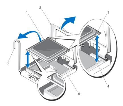
Figure 39. Removing and Installing a Processor
