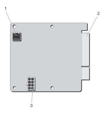
Figure 46. Power-Distribution Board Connectors
