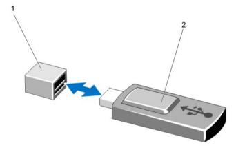
Figure 29. Replacing the Internal USB Key
