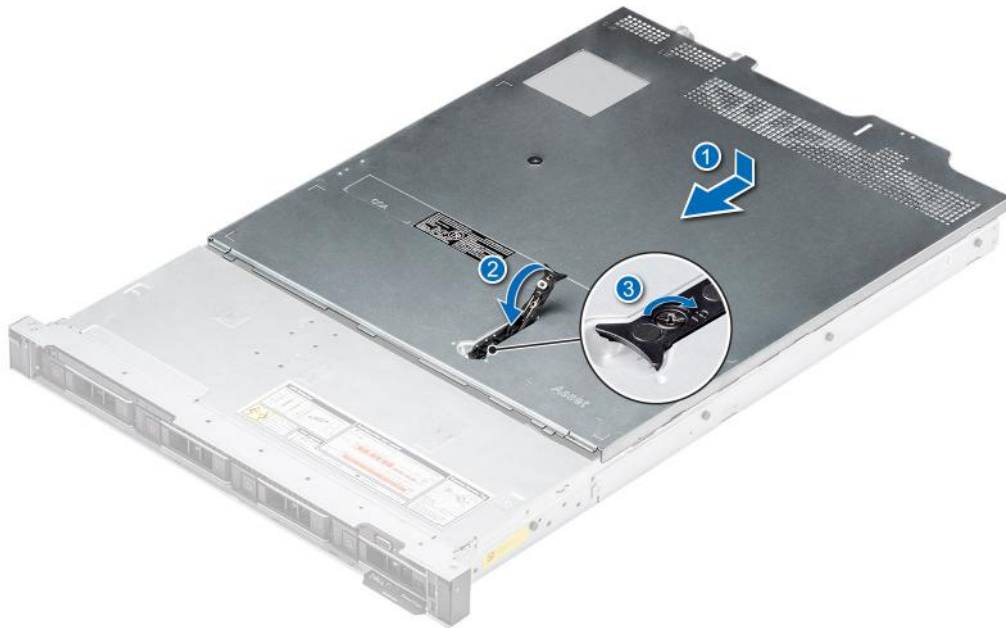
Figure 18. Installing the system cover
