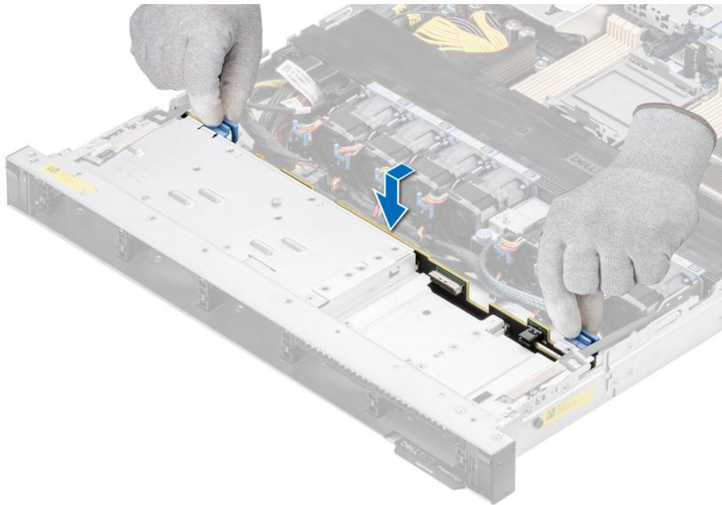
Figure 38. Installing the drive backplane
