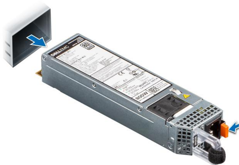
Figure 96. Removing a power supply unit
