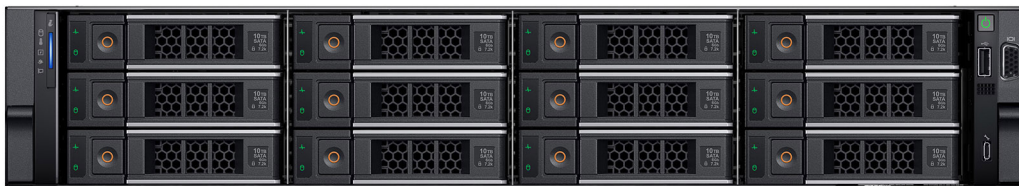
Figure 3. Front view of 12 x 3.5-inch SAS/SATA drive system
