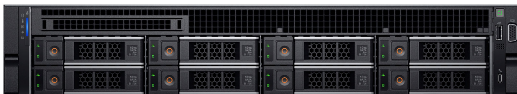
Figure 4. Front view of 8 x 3.5-inch SAS/SATA drive system
