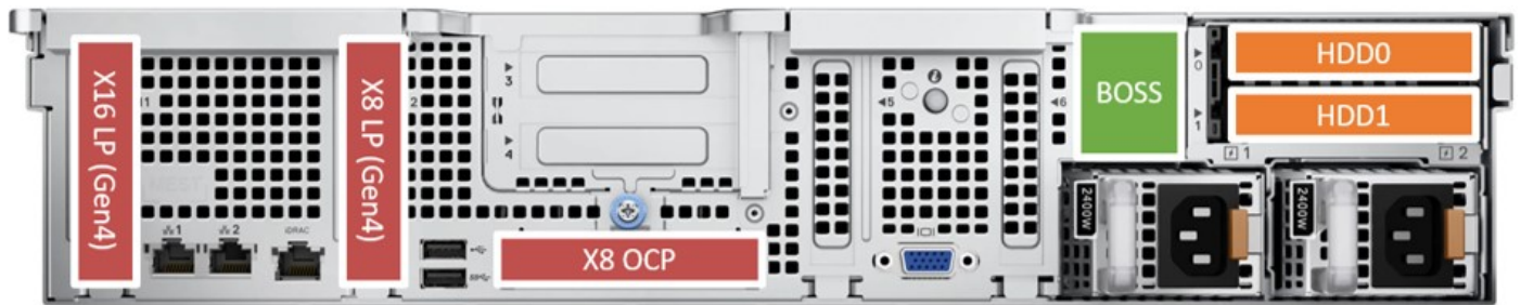
Figure 10. Rear view of the system with no riser and one CPU
