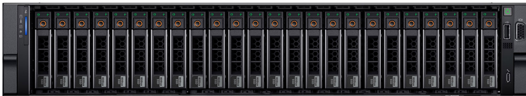
Figure 1. Front view of 16 x 2.5-inch SAS/SATA + 8 x 2.5-inch NVMe drive system
