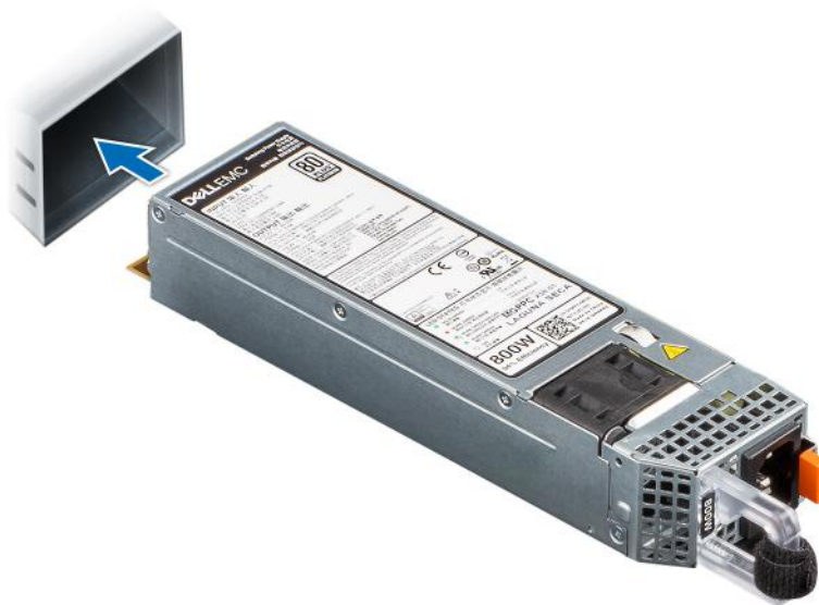
Figure 123. Installing a power supply unit
