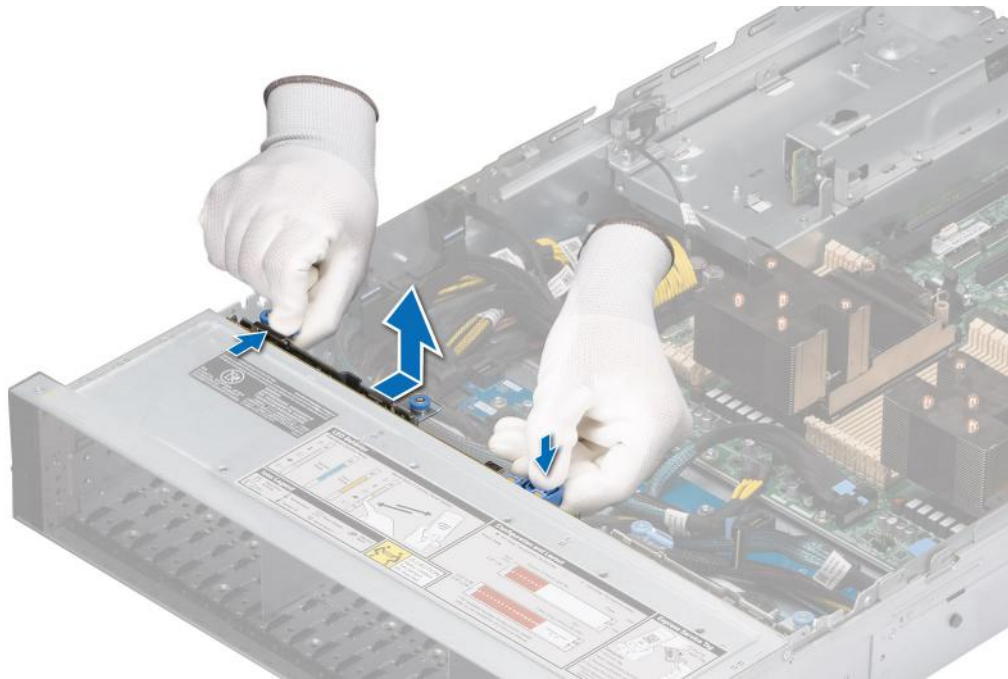
Figure 49. Removing the drive backplane
