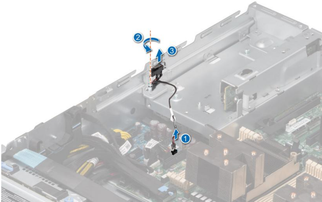
Figure 35. Removing the intrusion switch module
