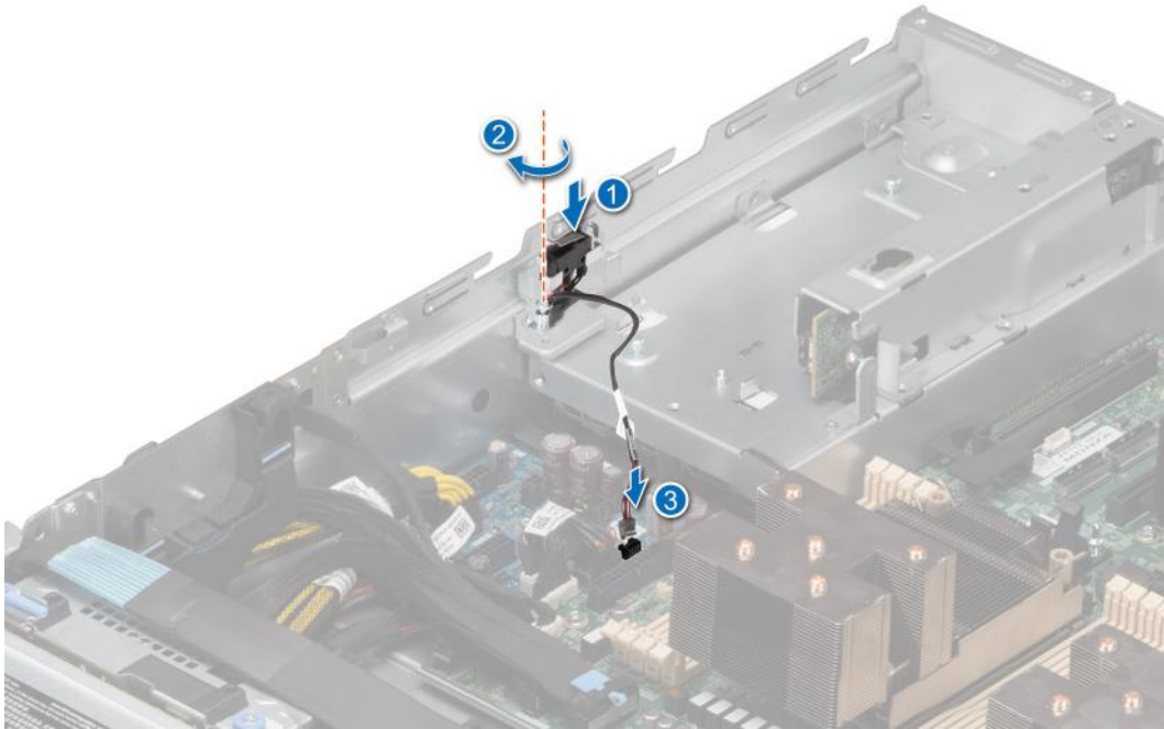
Figure 36. Installing the intrusion switch
