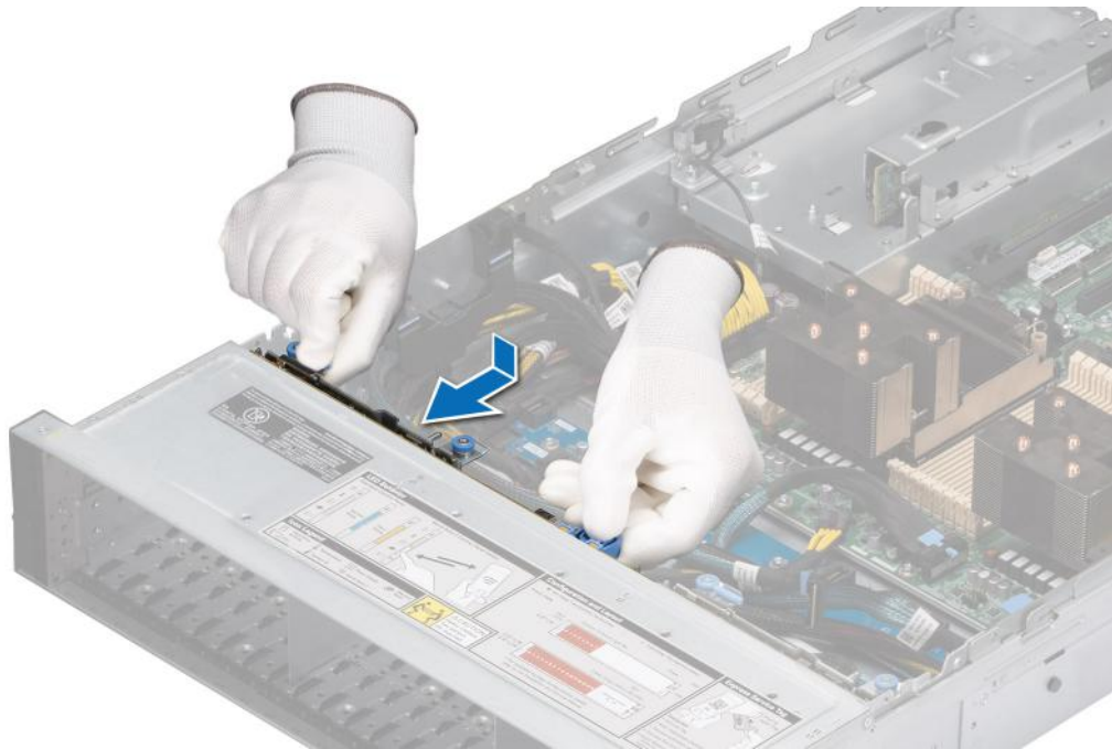
Figure 50. Installing the drive backplane
