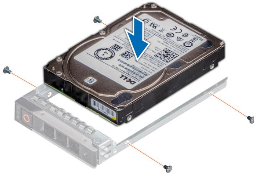
Figure 44. Installing a drive into the drive carrier
