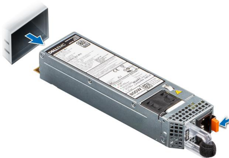
Figure 122. Removing a power supply unit
