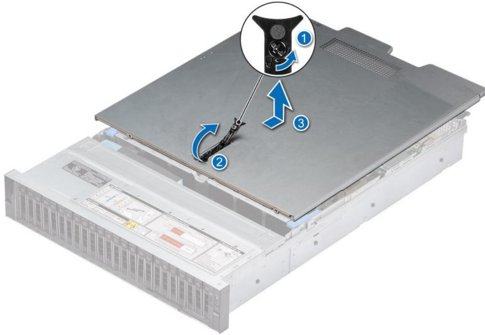
Figure 19. Removing the system cover
