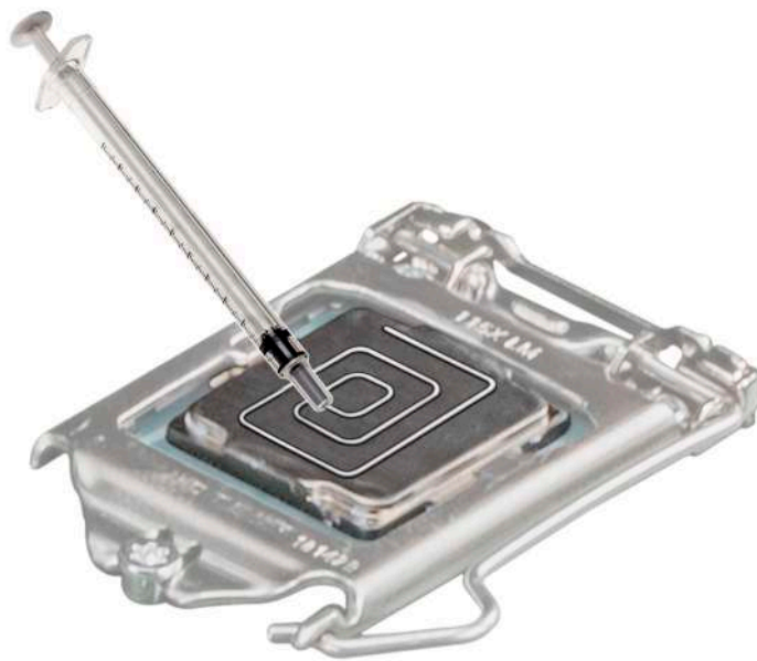
Figure 54. Applying thermal grease on top of the processor
