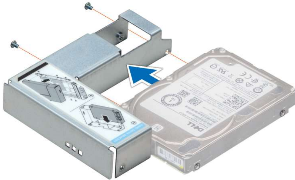
Figure 30. Installing a 2.5-inch drive into the 3.5-inch drive adapter
