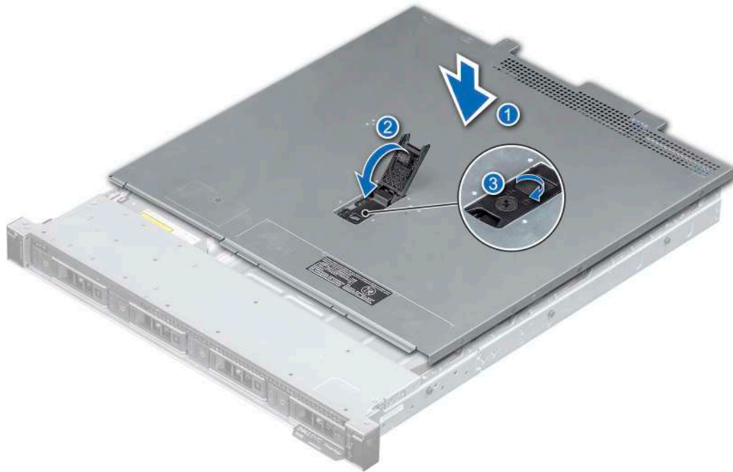
Figure 16. Installing the system cover
