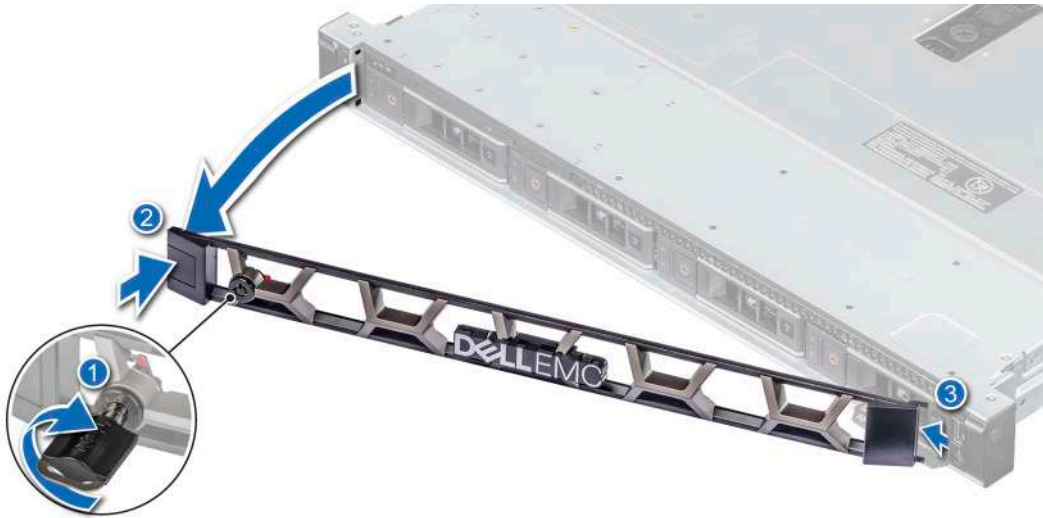
Figure 13. Removing the optional front bezel
