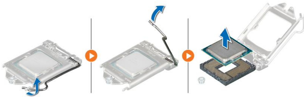
Figure 54. Removing the processor
