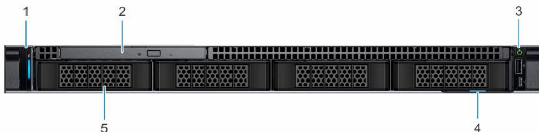
Figure 2. Front view of the 4 x 3.5-inch cabled drive system
