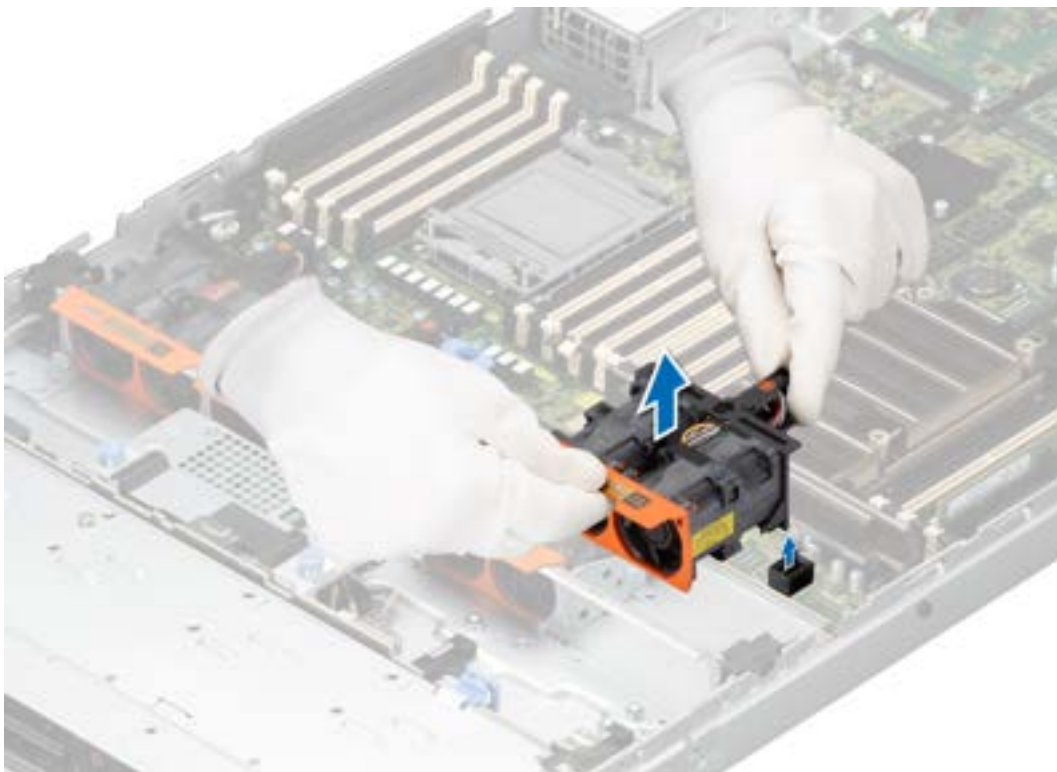
Figure 34. Removing a cooling fan module
