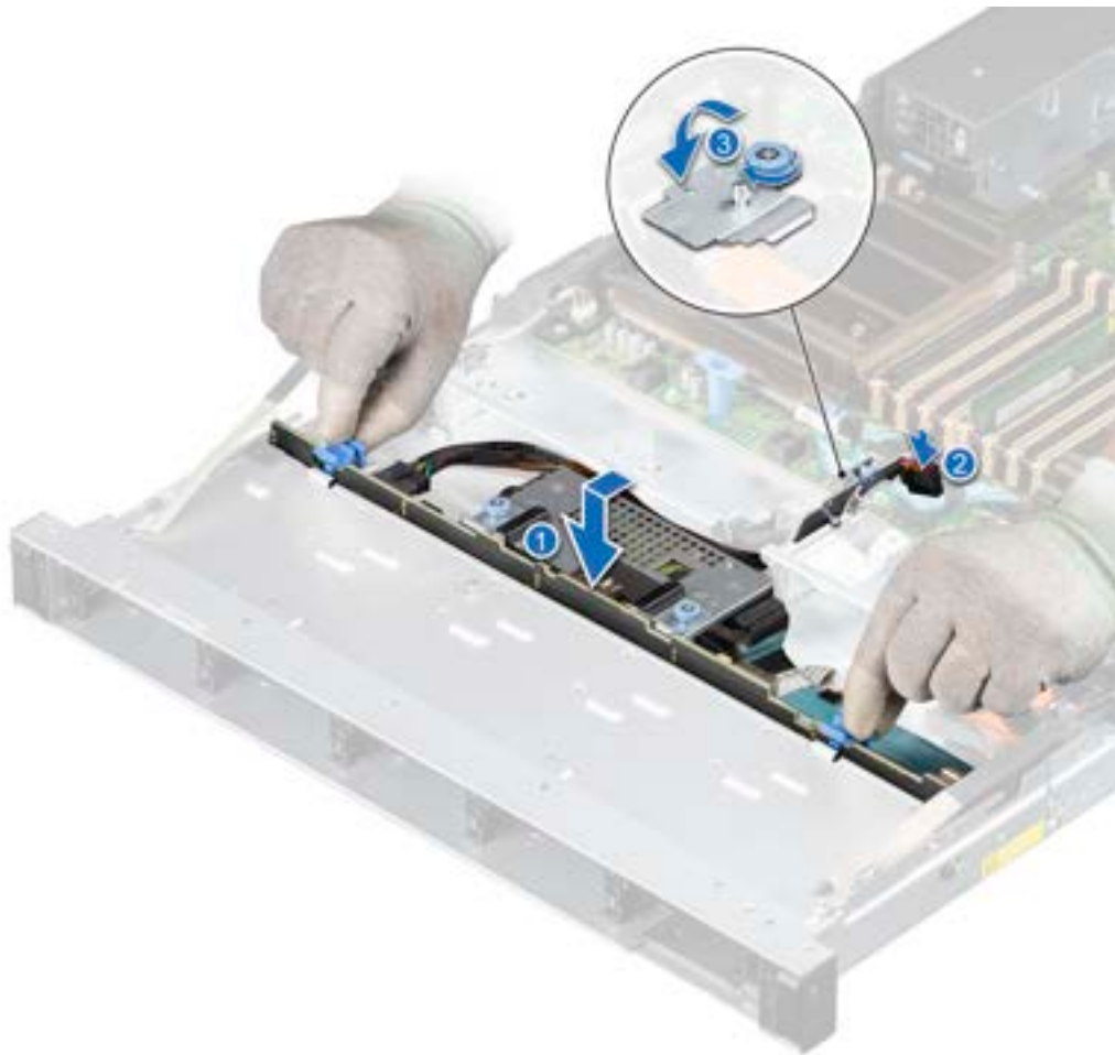
Figure 46. Installing the drive backplane
