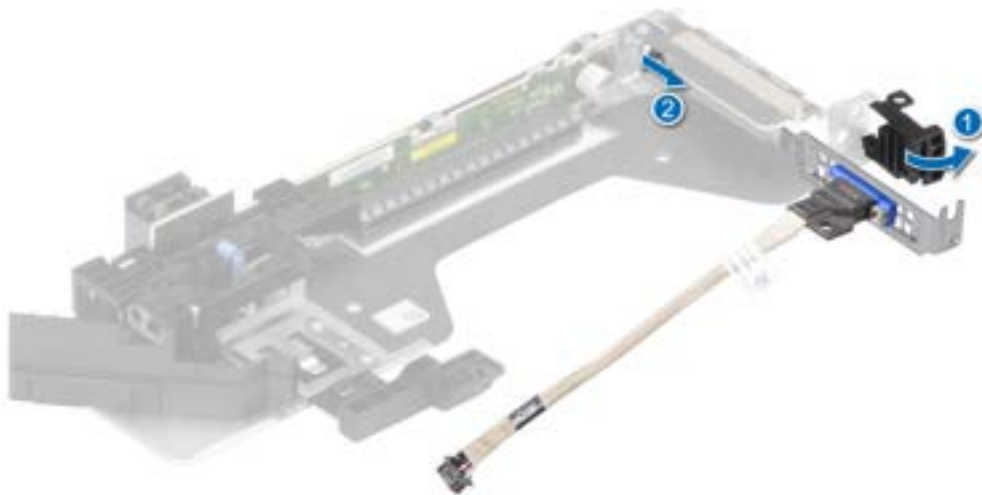
Figure 116. Removing the VGA port
