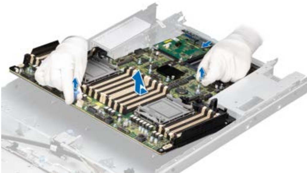
Figure 128. Removing the system board
