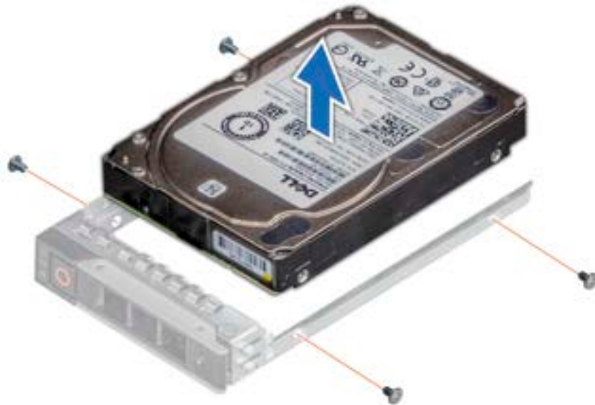
Figure 40. Removing the drive from the drive carrier
