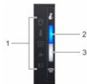
Figure 6. Left control panel with optional iDRAC Quick Sync 2.0 indicator
