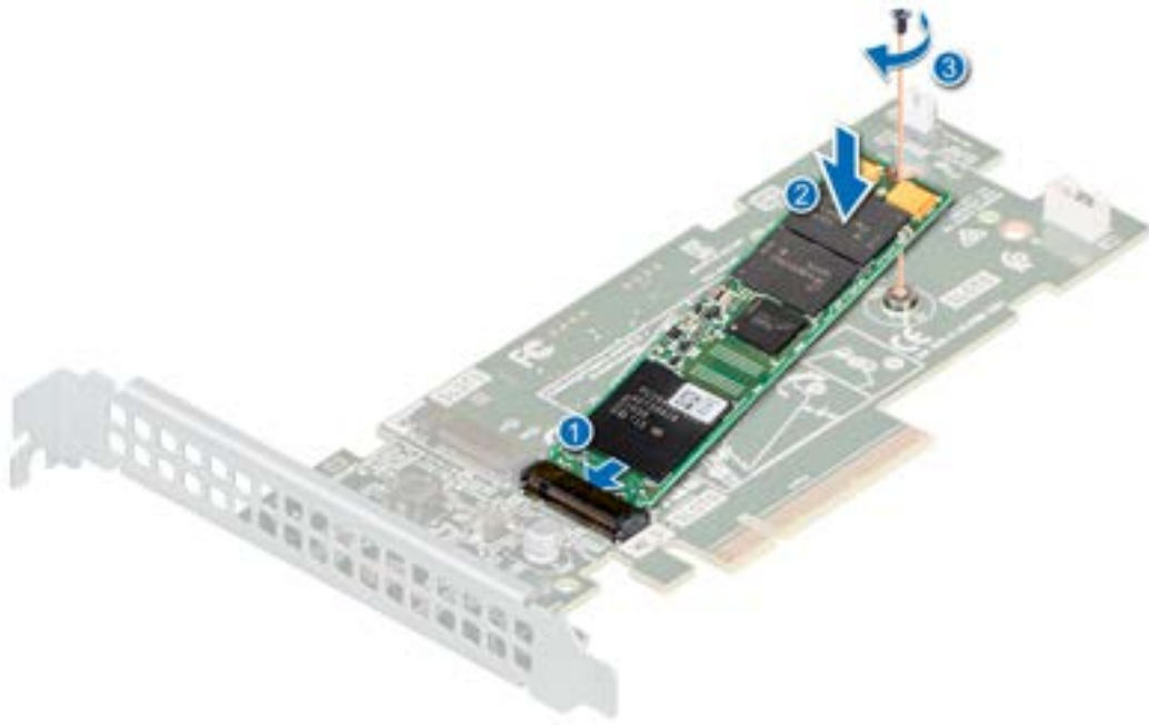
Figure 91. Installing the M.2 SSD module
