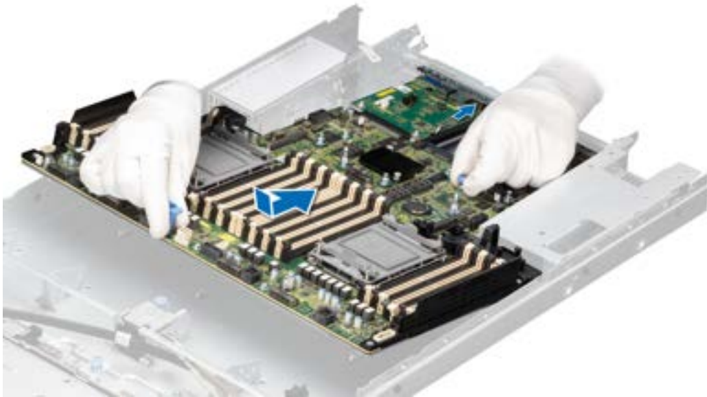
Figure 129. Installing the system board
