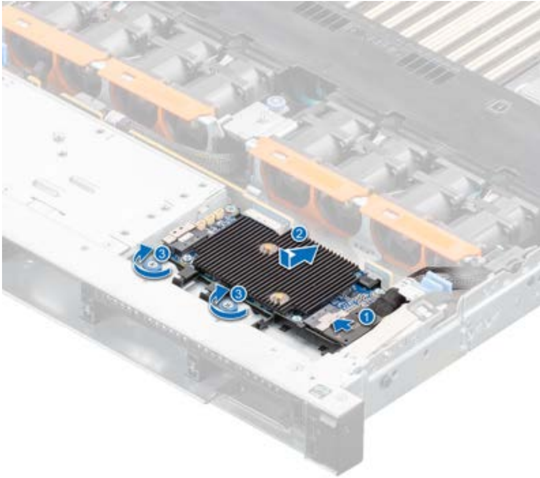
Figure 48. Installing the front mounting front PERC module
