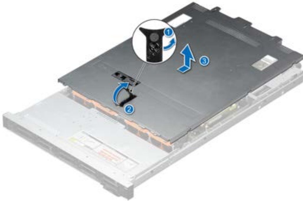
Figure 26. Removing the system cover
