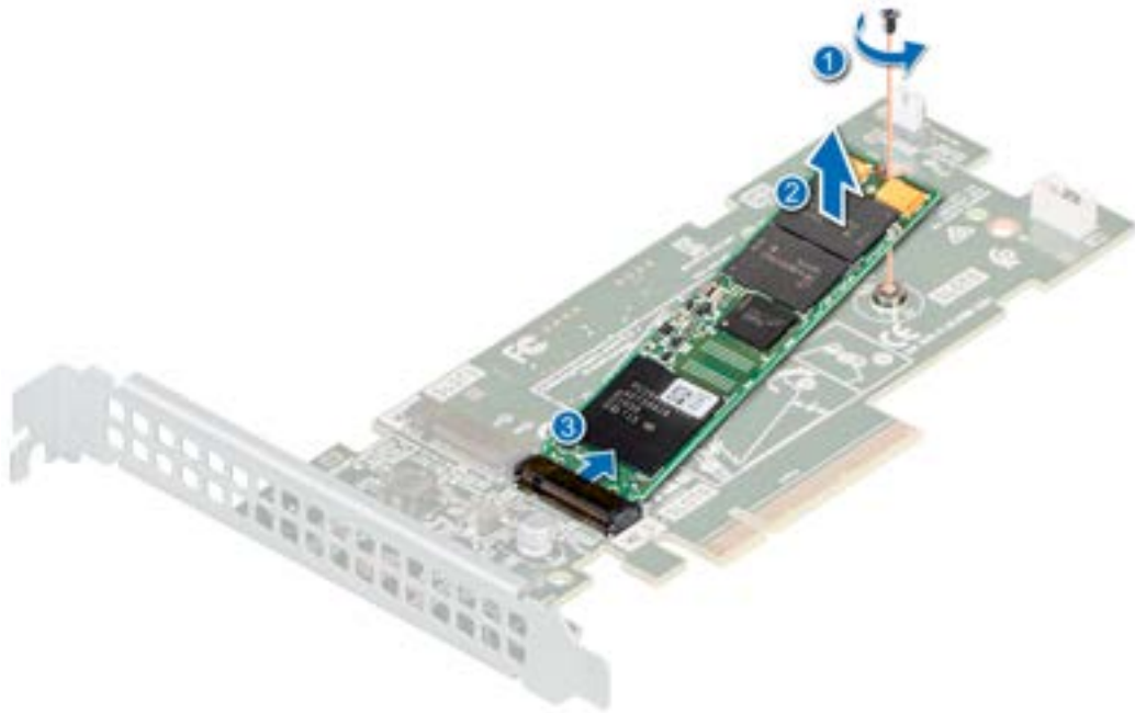
Figure 90. Removing the M.2 SSD module
