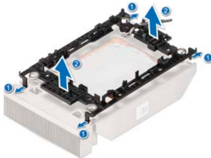
Figure 59. Removing the processor carrier
