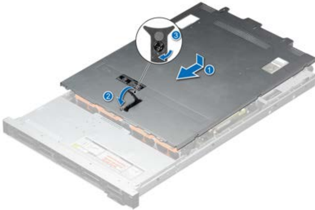
Figure 27. Installing the system cover
