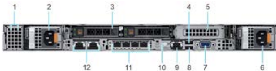
Figure 9. Rear view of the system with 2 x 2.5-inch rear drive module and 1 x LP PCIe slot
