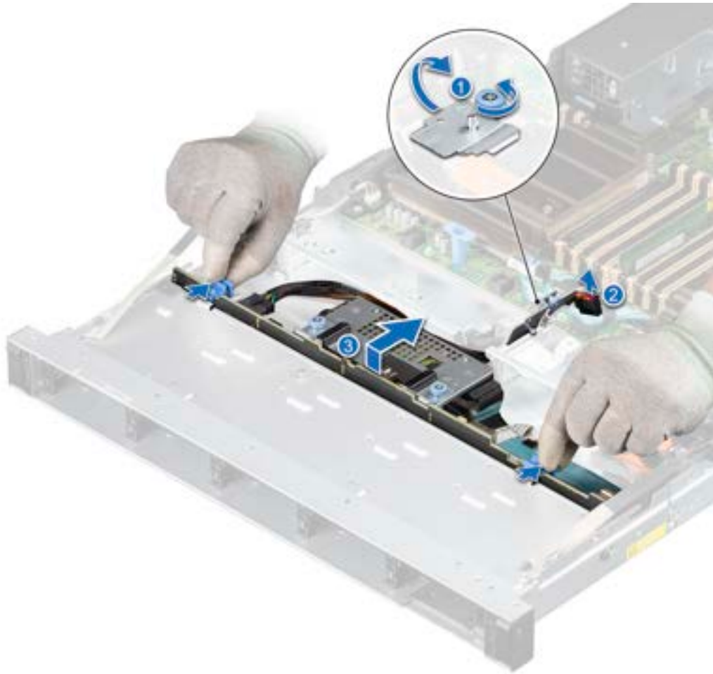
Figure 45. Removing the drive backplane
