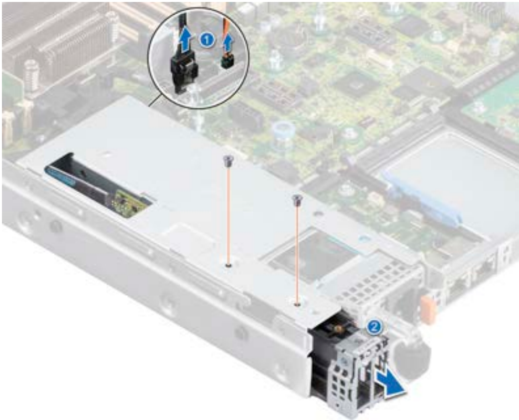
Figure 96. Removing the BOSS S2 module
