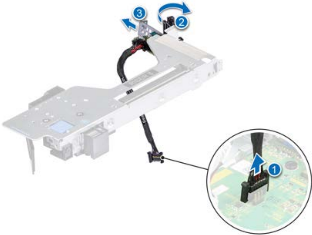
Figure 124. Removing the serial COM port
