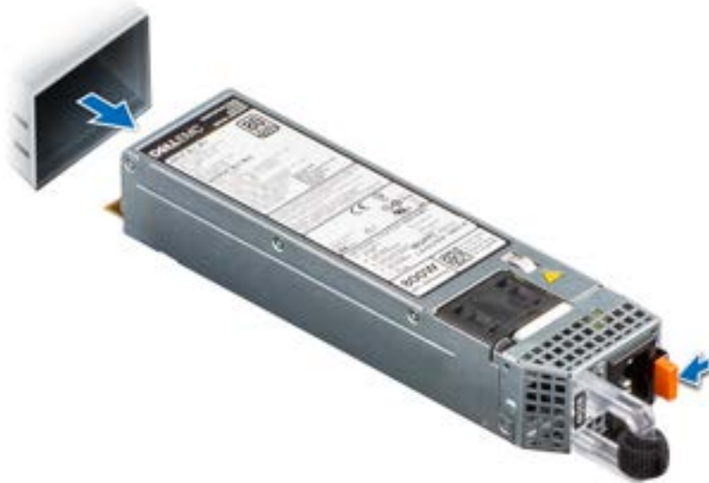
Figure 122. Removing a power supply unit
