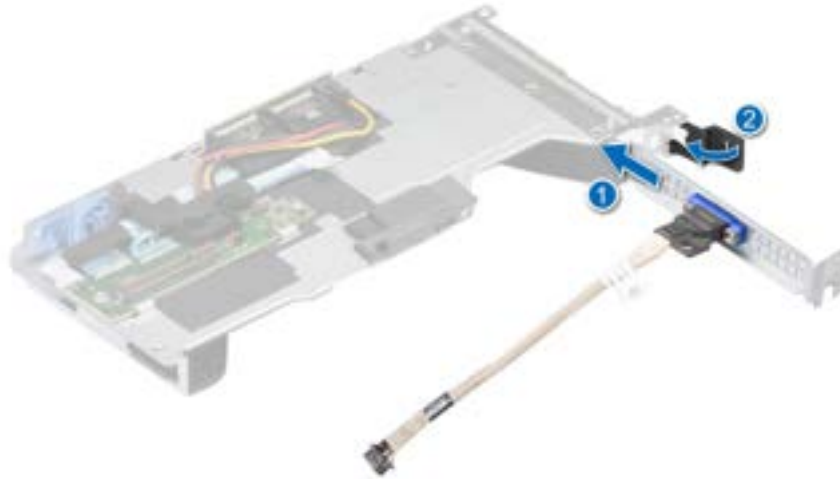
Figure 119. Installing the rear VGA port
