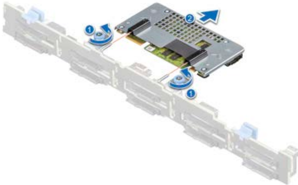
Figure 49. Removing the rear mounting front PERC module
