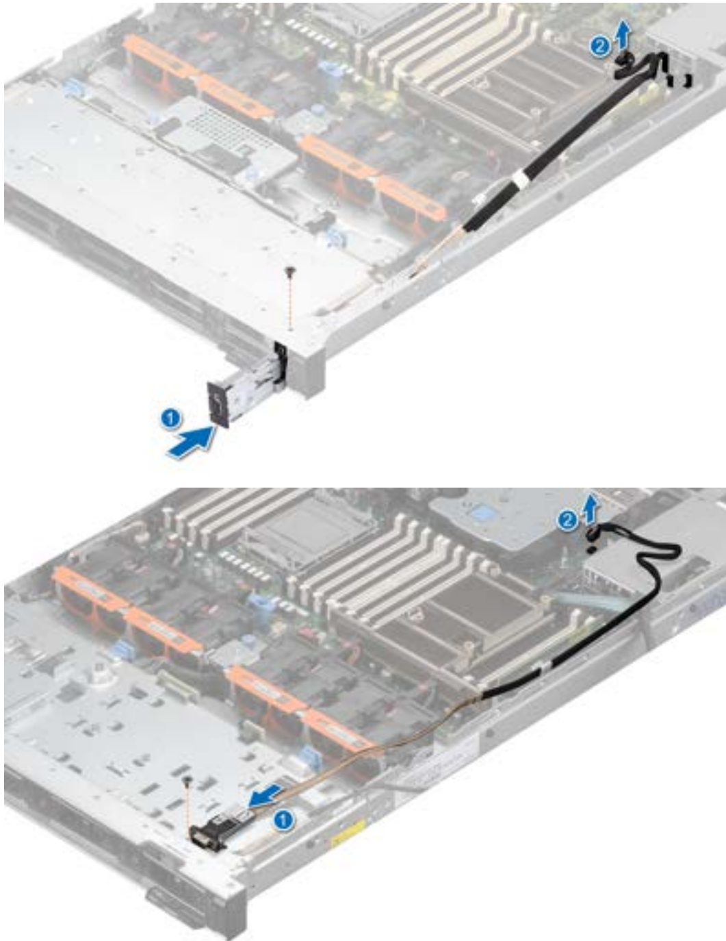
Figure 115. Installing the VGA module
