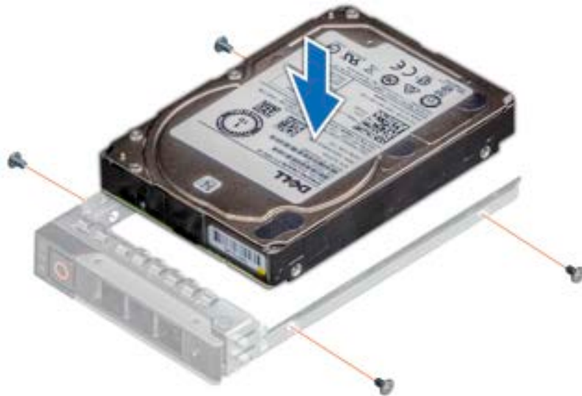
Figure 41. Installing a drive into the drive carrier
