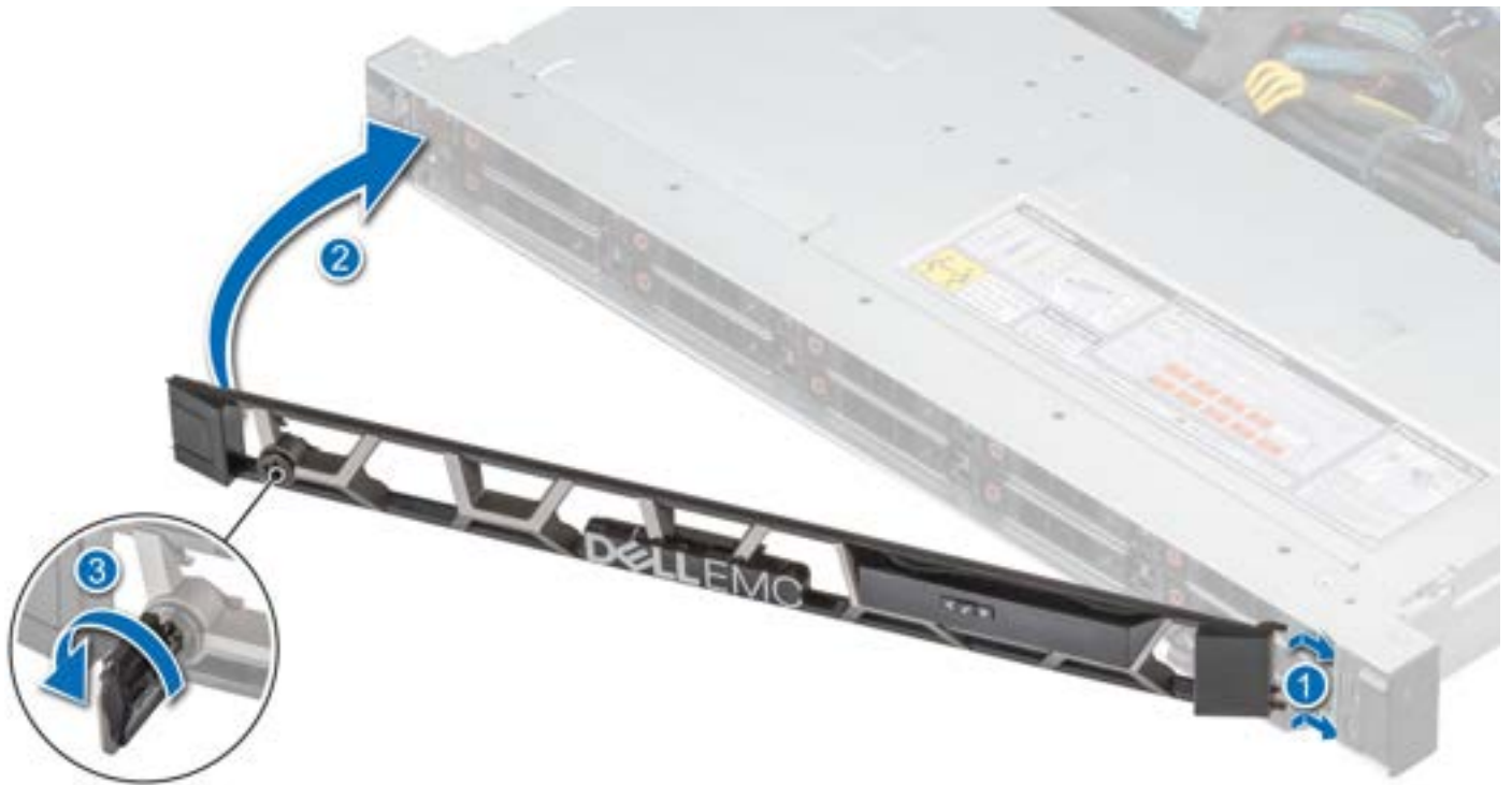
Figure 25. Installing the front bezel with the LCD panel
