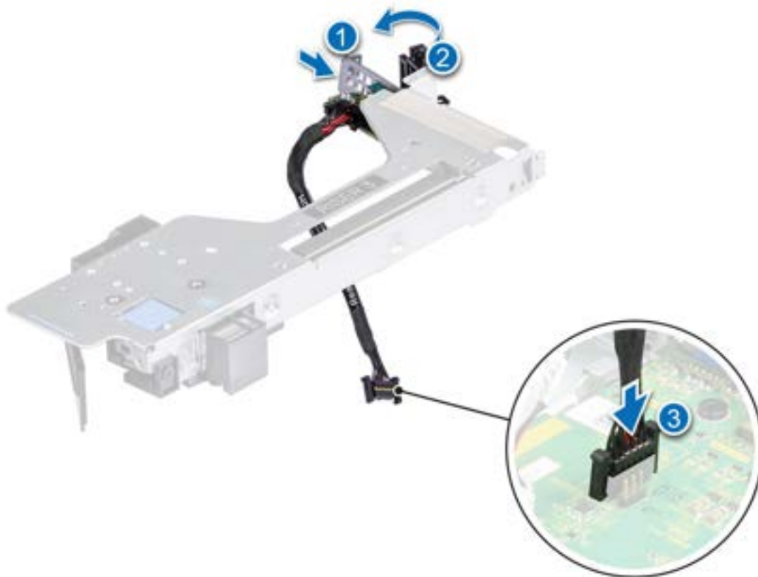
Figure 127. Installing the serial COM port
