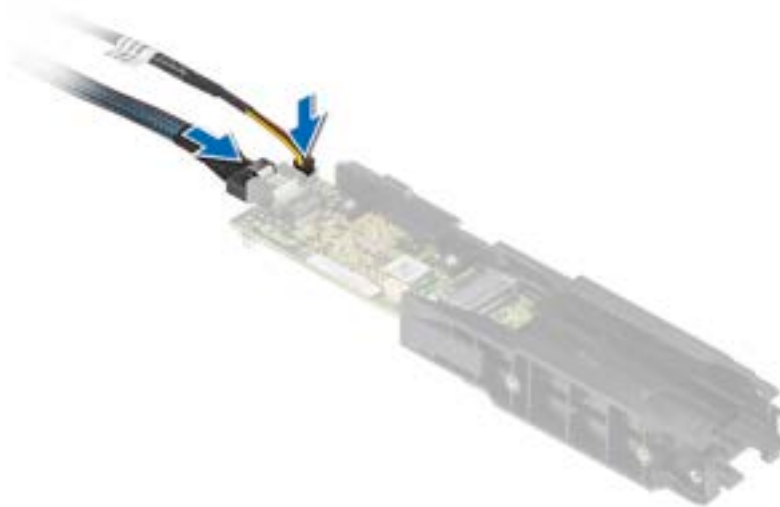
Figure 100. Connecting the BOSS power cable and BOSS Signal cable to the BOSS S2 module
