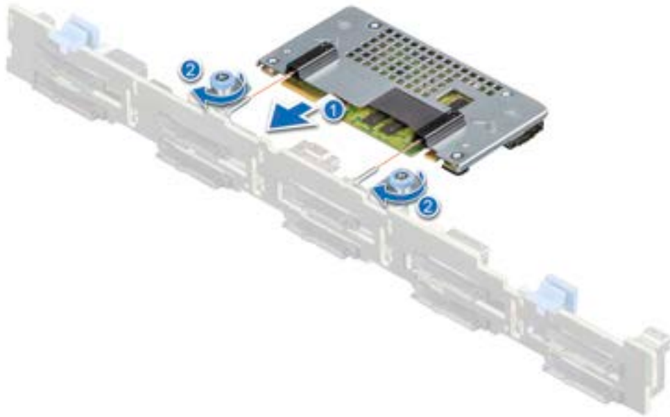
Figure 50. Installing the rear mounting front PERC module
