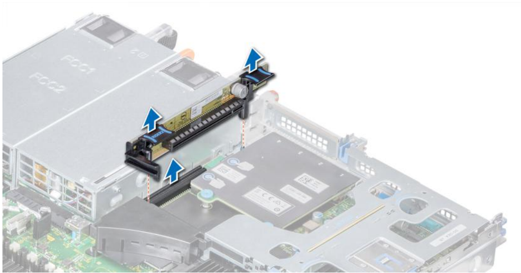
Figure 48. Removing the expansion riser 2A
