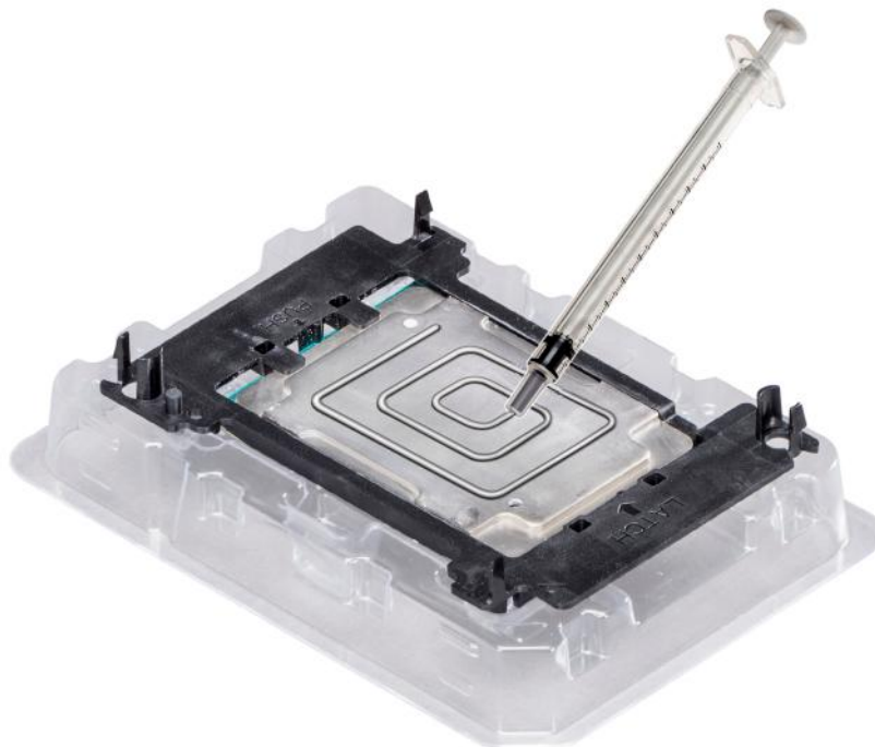
Figure 43. Applying thermal grease on top of the processor
