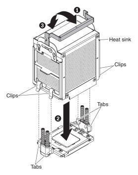
15. Press on the top of the heat sink and rotate the lever to the closed position.
