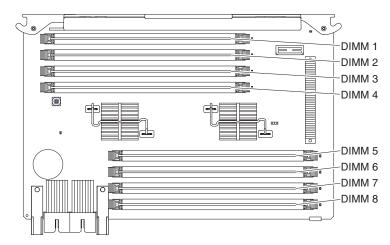
• In a low-cost and low-power DIMM installation, install the DIMMs on each memory card in the order shown in the following tables. The goal in a low-cost and low-power configuration is to completely fill each memory card before you install the next memory card.
