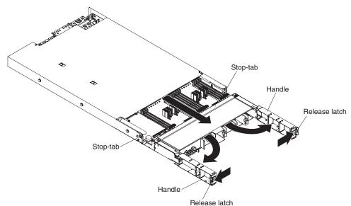
5. Grasp the handles and pull the system-board tray out until it stops; then, press in the blue stop-tabs on both sides of the system-board tray and pull the tray out of the chassis.
