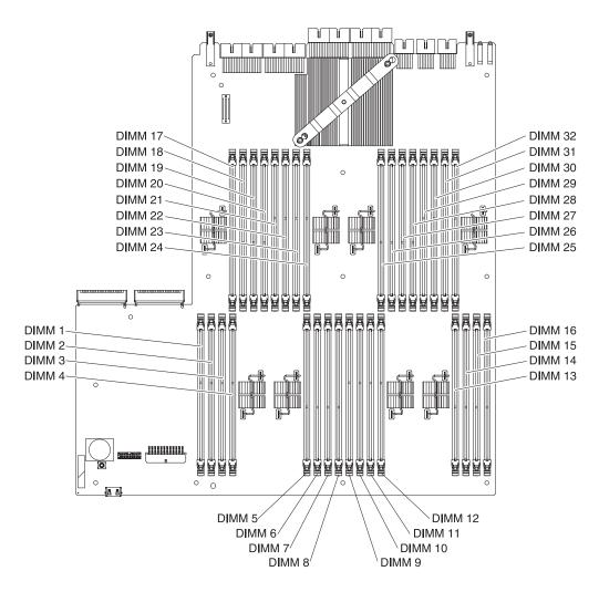
To install a DIMM (memory module) in the memory expansion module, complete the following steps.
