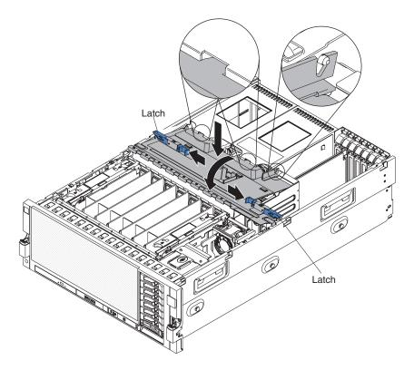
To replace the top-cover bracket, complete the following steps:
