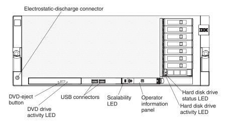
**Electrostatic-discharge connector:** Connect a electrostatic-discharge wrist strap to this connector when you work with static-sensitive devices.
