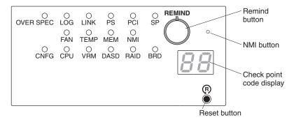
• **Remind button:** This button places the system-error LED on the front panel into Remind mode. In Remind mode, the system-error LED flashes once every 2 seconds until the problem is corrected, the server is restarted, or a new problem occurs.
