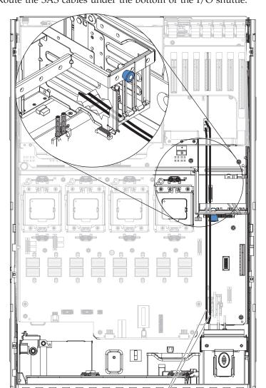
11. Route the SAS cables under the bottom of the I/O shuttle.
