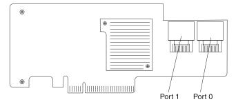
**18**. Install the ServeRAID adapter onto the RAID adapter carrier, and then install the carrier into the server.
