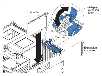
6. Remove the expansion-slot cover.
