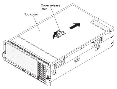
4. Lift the cover-release latch. The cover slides to the rear approximately 13 mm (0.5 inch). Lift the cover off the server.
