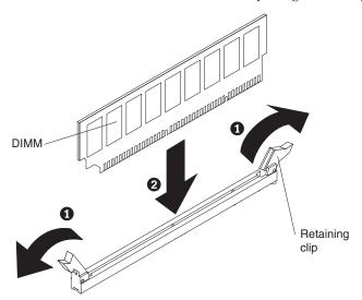
9. Insert the DIMM into the connector by aligning the edges of the DIMM with the slots at the ends of the DIMM connector. Firmly press the DIMM straight down into the connector 2 by applying pressure on both ends of the DIMM simultaneously. The retaining clips snap into the locked position when the DIMM is seated in the connector.
