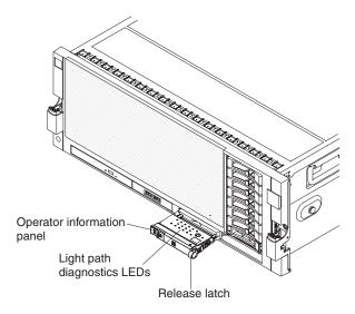
The following illustration shows the controls and LEDs on the light path diagnostics panel.
