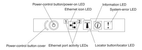
The following controls and LEDs are on the operator information panel:
