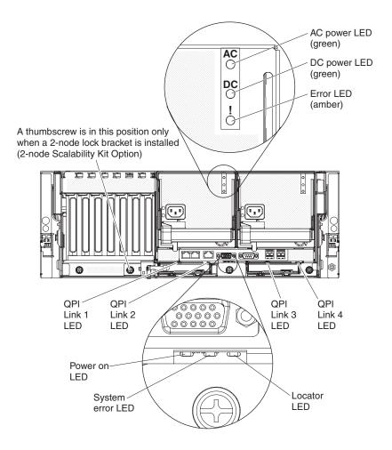
**AC power LED:** Each hot-swap power supply has an ac power LED and a dc power LED. When the ac power LED is lit, it indicates that sufficient power is coming into the power supply through the power cord. During typical operation, both the ac and dc power LEDs are lit. For any other combination of LEDs, see the *Problem Determination and Service Guide*.
