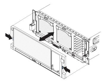
**Note:** You do not have to remove the top cover before you remove the bezel.
