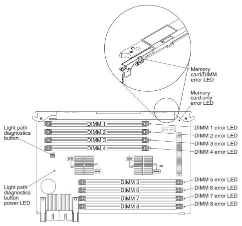
**Memory card/DIMM error LED:** When this LED is lit, it indicates that the memory card or a DIMM has failed.
