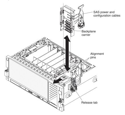
**6**. Disconnect the power and configuration cables from the backplane. Do not disconnect the SAS signal cable from the backplane.
