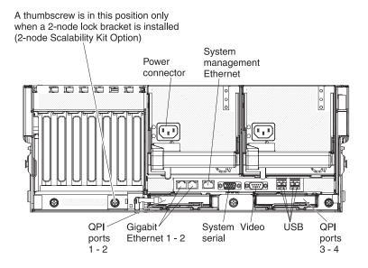
**Power-cord connector:** Connect the power cord to this connector.
