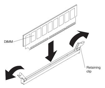
10. Firmly press the DIMM straight down into the connector by applying pressure on both ends of the DIMM simultaneously. The retaining clips snap into the locked position when the DIMM is firmly seated in the connector.
