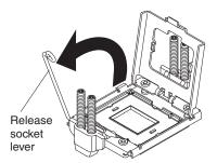
8. Remove the socket cover from the microprocessor socket. The microprocessor socket might have the socket cover style shown in illustration A or the style shown in illustration B.
