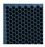
In addition, the server uses **hexagonal ventilation holes** in the chassis. Hexagonal holes can be grouped more densely than round holes, providing greater airflow through the system cover.
