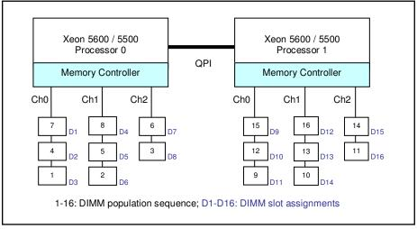
This new processor design comes with some trade-offs in memory capacity, performance, and cost: For example, **greater memory capacity** comes with **lower memory speed**. Alternatively, it is possible to achieve the **same memory capacity at lower cost** but **at a lower memory speed**.
