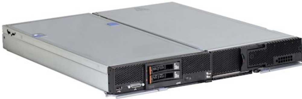
Figure 5. Flex System Storage Expansion Node (right) attached to a compute node (left)
