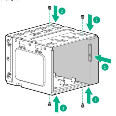
11. Install the non-hot-plug drive cage.
