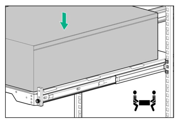
3. Press and hold the blue rail-release tabs (callout 1), and then slide the tray back into the rack (callout 2).
