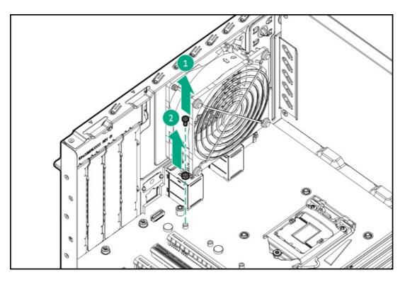
b. Install the removed hex nut on the 2280 standoff.
