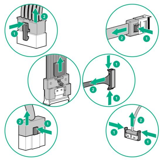
Remove cables that are no longer being used. Retaining them inside the system can restrict airflow. If you intend to use the removed cables later, label and store them for future use.
