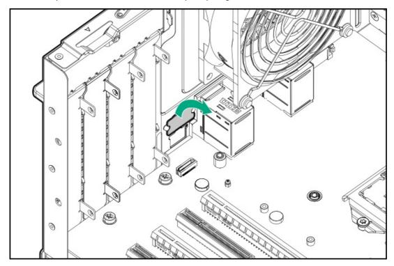
Remove the SSD mounting screw and hex nut from the 22110 standoff on the system board.
