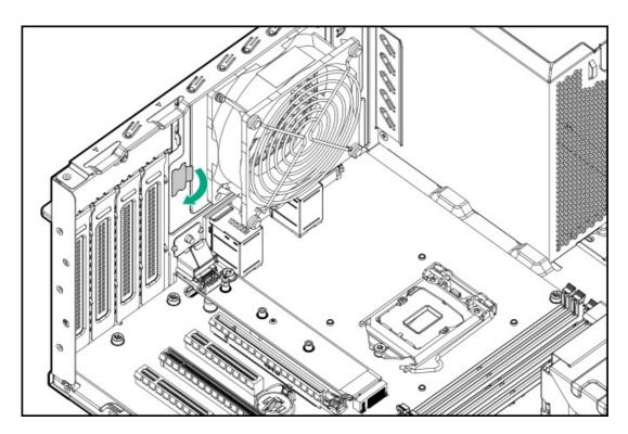
17. Install the serial port cable clip.
