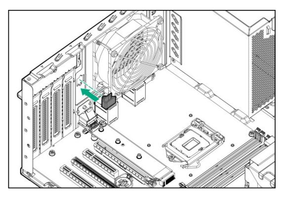
18. Connect the serial port cable, and then secure the extra length of the cable in the serial port cable clip .
