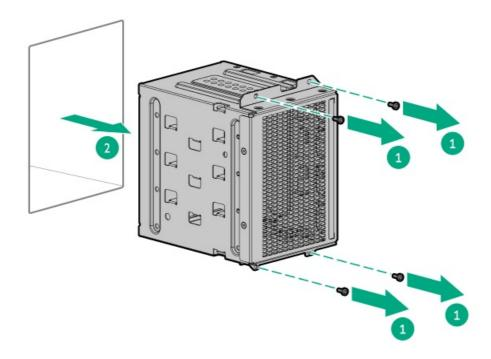
9. Remove the correct number of screws from the drive cage.
