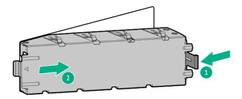
9. Install the optical drive bracket.
