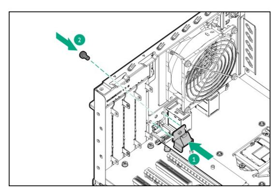
11. If no M.2 SSD will be installed on the iLO-M.2-serial module, install the SSD mounting screw and hex nut removed on <a href="step 9">step 9</a> on the <a href="M.2 22110 standoff">M.2 22110 standoff on the module</a>.
