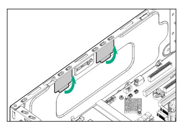
b. Insert the holder tabs into their corresponding chassis slots.
