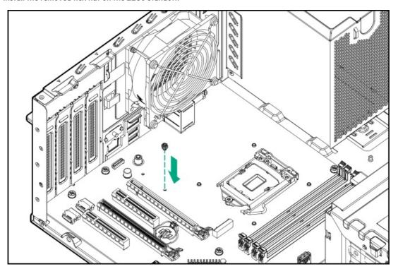
8. If you are installing an M.2 22110 SSD, remove the SSD mounting screw from the 22110 standoff.
