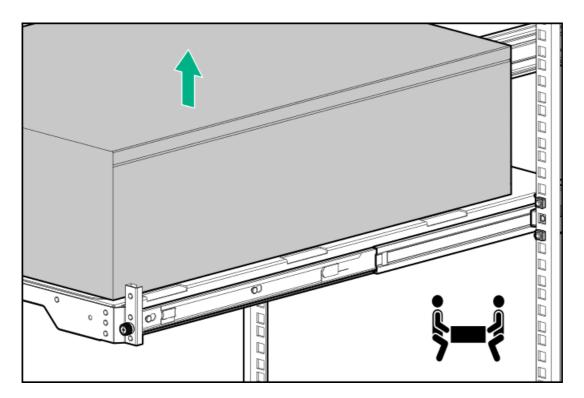
7. Place the server on a flat, level surface with the access panel facing up.
