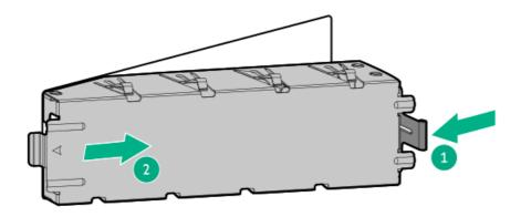
9. Secure the metal shims on the LTO tape drive.
