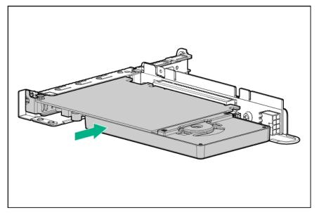
7. Install the GPU support bracket.
