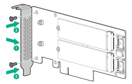
7. Remove the expansion slot cover.
