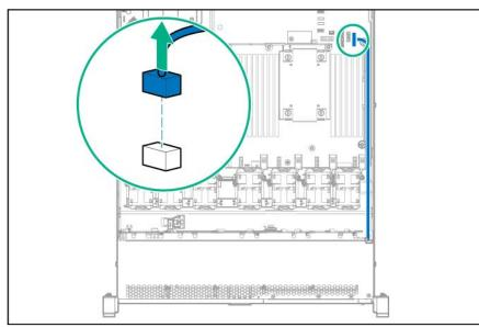
6. Remove the Power/UID/USB assembly.
