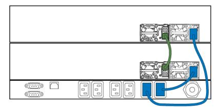
6. Charge the FSBBU module until the LED is solid green.
