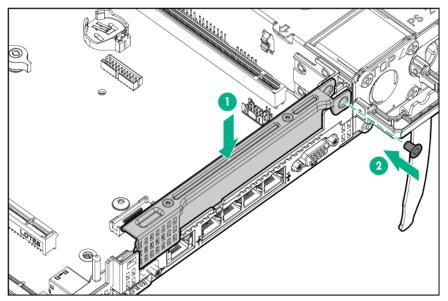
9. Align the PCIe x16 riser cage with the corresponding connector on the system board, and then press down on the riser cage.
