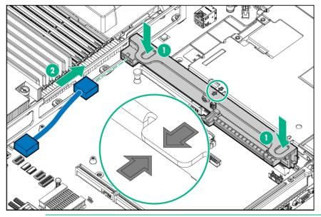
**CAUTION:** To prevent improper cooling and thermal damage, do not operate the server unless all PCI slots have either an expansion slot cover or an expansion board installed.
