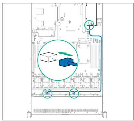
**9.** If the 2SFF SAS/SATA backplane is installed, connect the Mini-SAS cable from the optional backplane to port 2 on the P840 controller board.
