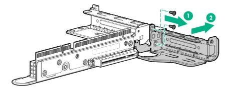
7. Lift and remove the riser cage latch.
