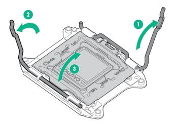
7. Remove the clear processor socket cover. Retain the processor socket cover for future use.
