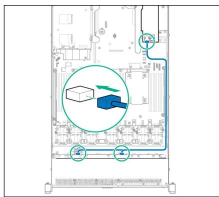
2. If the 2SFF SAS/SATA backplane is installed, connect the Mini-SAS cable from the optional backplane to port 2 on the P840 controller board.
