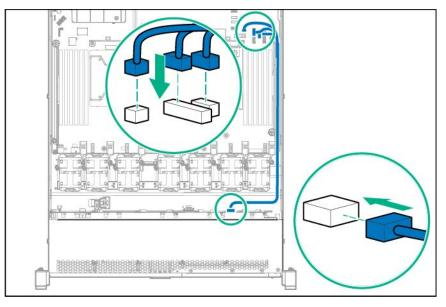
2. Connect the power cable to the left power connector on the backplane.
