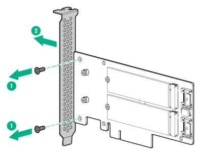
**b.** Install the low-profile bracket on the M.2 SSD enablement board.
