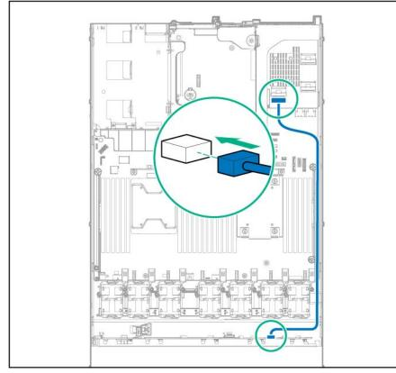
**13.** Connect the power cable to the left power connector on the backplane.
