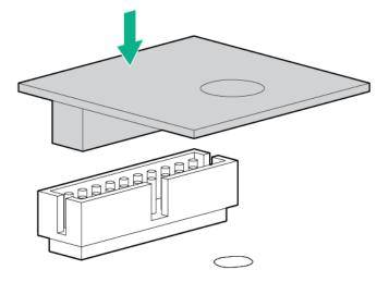
7. Install the TPM security rivet by pressing the rivet firmly into the system board.
