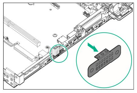
6. Connect the serial cable option. Then, remove the backing from the double-sided tape and press down where indicated.
