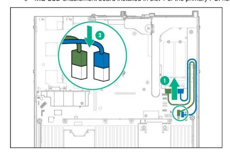
o M.2 SSD enablement board installed in slot 3 of the secondary PCI riser
