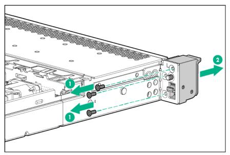
6. Install the location discovery services ear option and route the location discovery services cable through side channel.
