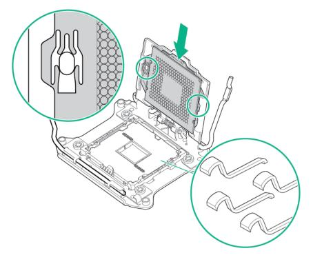
9. Close the processor retaining bracket. When the processor is installed properly inside the processor retaining bracket, the processor retaining bracket clears the flange on the front of the socket.
