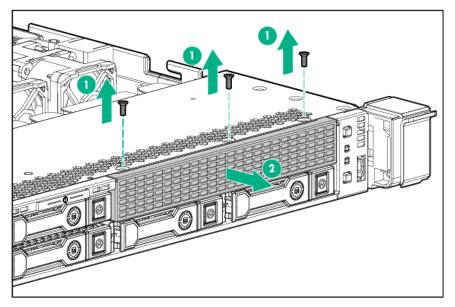
6. Install the drive cage assembly, and then tighten the three screws.
