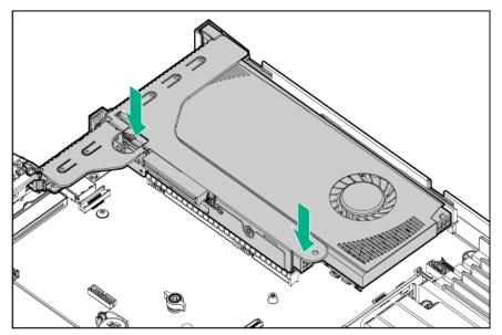
9. Connect the GPU riser cable to the GPU and the primary riser cage PCA.
