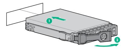
4. Install an SFF drive blank in any unused drive bays.
