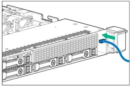
2. Install the SID module into the front panel and secure the module to the chassis with the screws from the kit.
