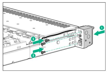
7. Install the discovery cable protection panel.
