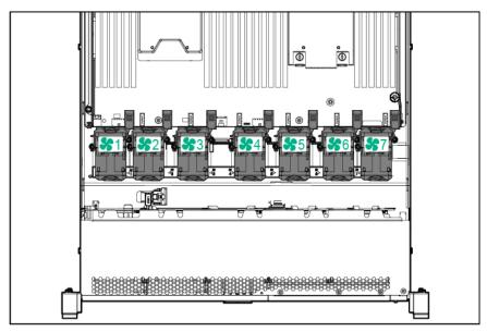
For a single-processor configuration, five fans and two blanks are required in specific fan bays for redundancy.
