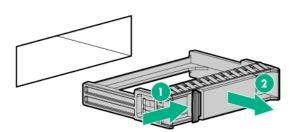
2. Press the Do Not Remove button to open the release handle.
