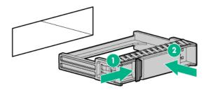
**CAUTION:** Do not remove an NVMe SSD from the drive bay while the Do Not Remove button LED is flashing. The Do Not Remove button LED flashes to indicate the device is still in use. Removal of the NVMe SSD before the device has completed and ceased signal/traffic flow can cause loss of data.
