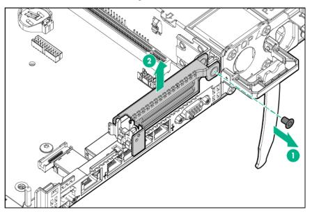
8. Install the full height PCIe x16 riser cage latch.
