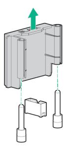
4. Remove the location discovery cable protection panel from the left side of the server.
