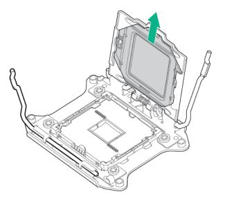
CAUTION: THE PINS ON THE SYSTEM BOARD ARE VERY FRAGILE AND EASILY DAMAGED. To avoid damage to the system board, do not touch the processor or the processor socket contacts.
