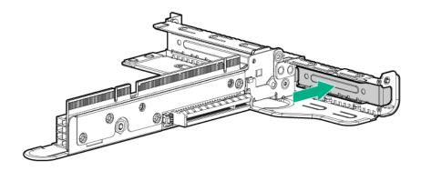
The controller board can be installed in slot 1 or slot 2.
