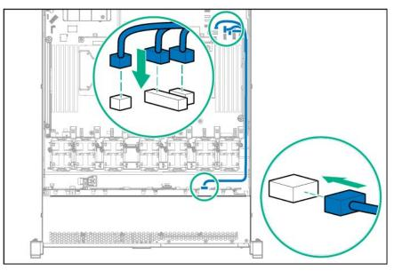
8. Connect the power cable to the left power connector on the backplane.
