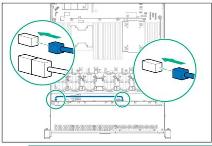
**NOTE:** Cabling from the 2SFF SAS/SATA backplane will vary if a PCIe storage controller is installed.
