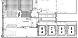
1-6 Non-hot plug LFF SATA hard drive bays - Using quick release carrier (LFF SAS supports 1-4 only)
