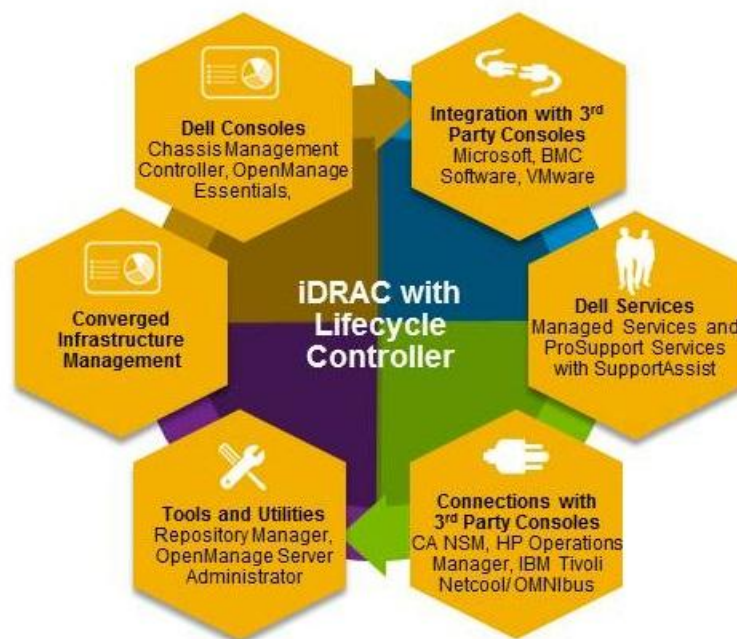
Figure 10. Dell systems management solutions
