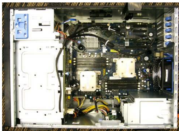
Figure 13. Hot-swap Hard Disk Drives Configuration without Air Shroud
