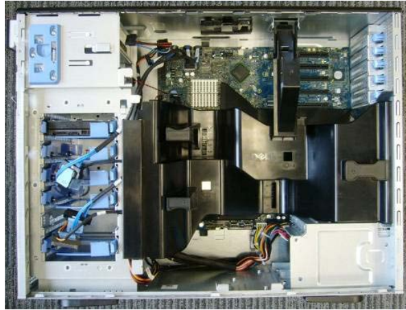
Figure 11. Cabled HDD Configuration with Air Shroud
