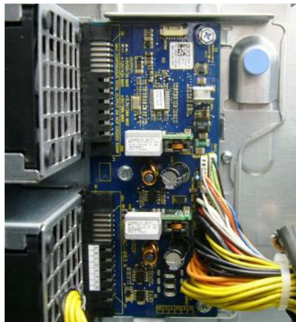
Figure 15. Power Distribution Board (PDB) for Redundant PSU
