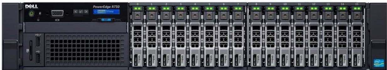
Figure 2. R730 front view (2.5" chassis without bezel)
